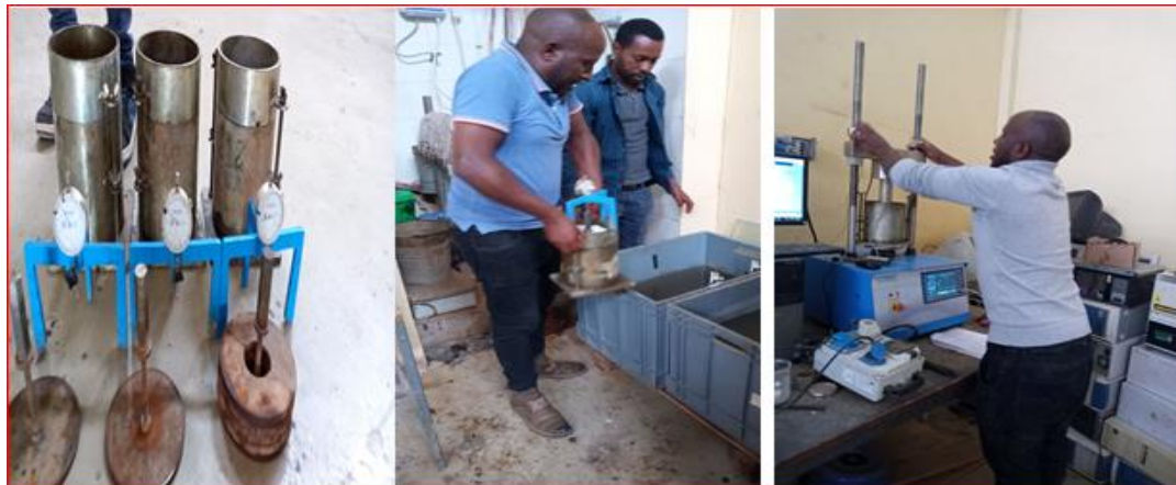
Figure 4.9 Soaked CBR Procedures (16/10/2021 & 20/10/2021)
