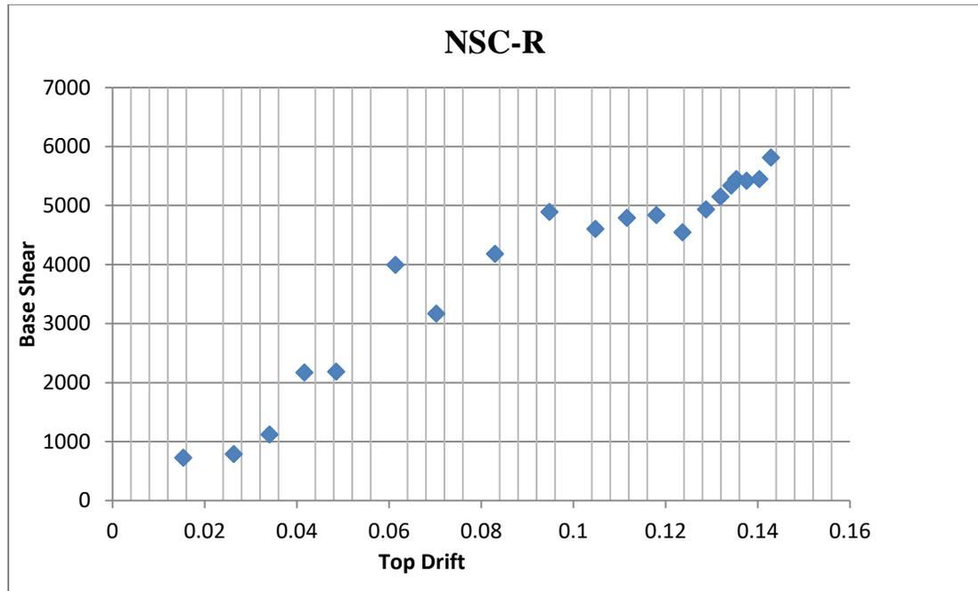
Figure 6.11: IDA capacity curve for NSC-R MRF
