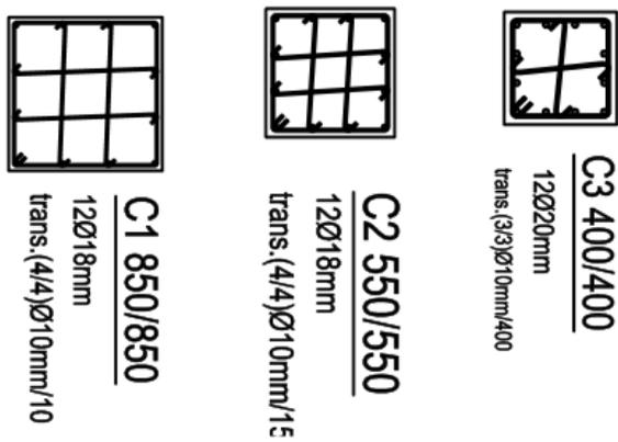
Figure 5.1: NSC-R moment resisting frame (MRF) reinforcement detail
