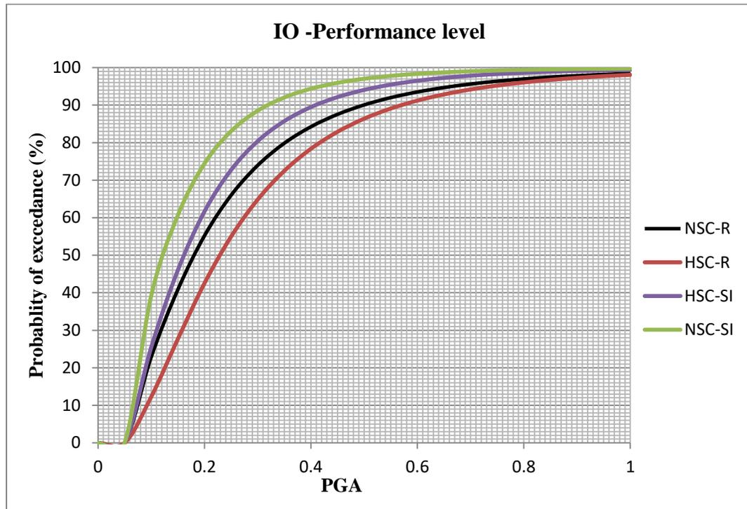
Figure 6.20: Fragility curve of both regular and stiffness irregular for IO Level
