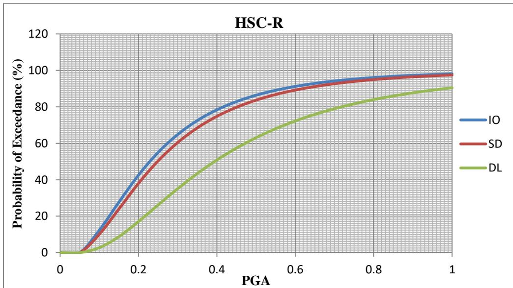
Figure F.2: Fragility curve of HSC-R MRF
