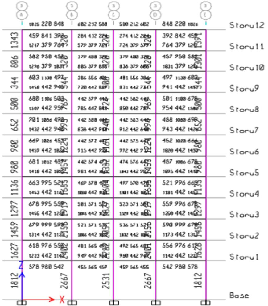
Figure B.3 NSC-SI frame design values from ETABS v-18.1
