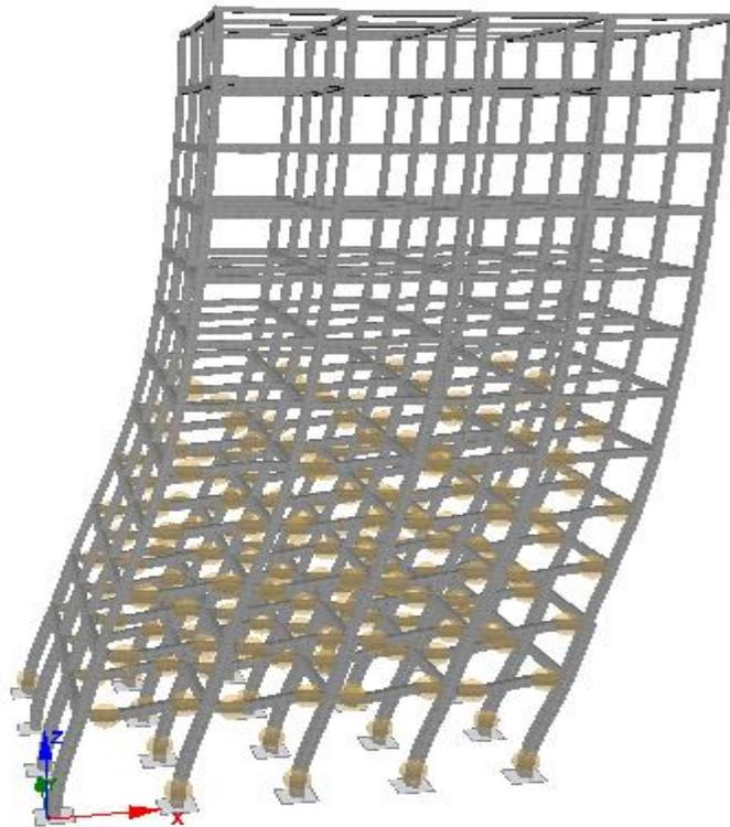
Figure 6.8: Deformed shape and plastic formation for HSC-SI
