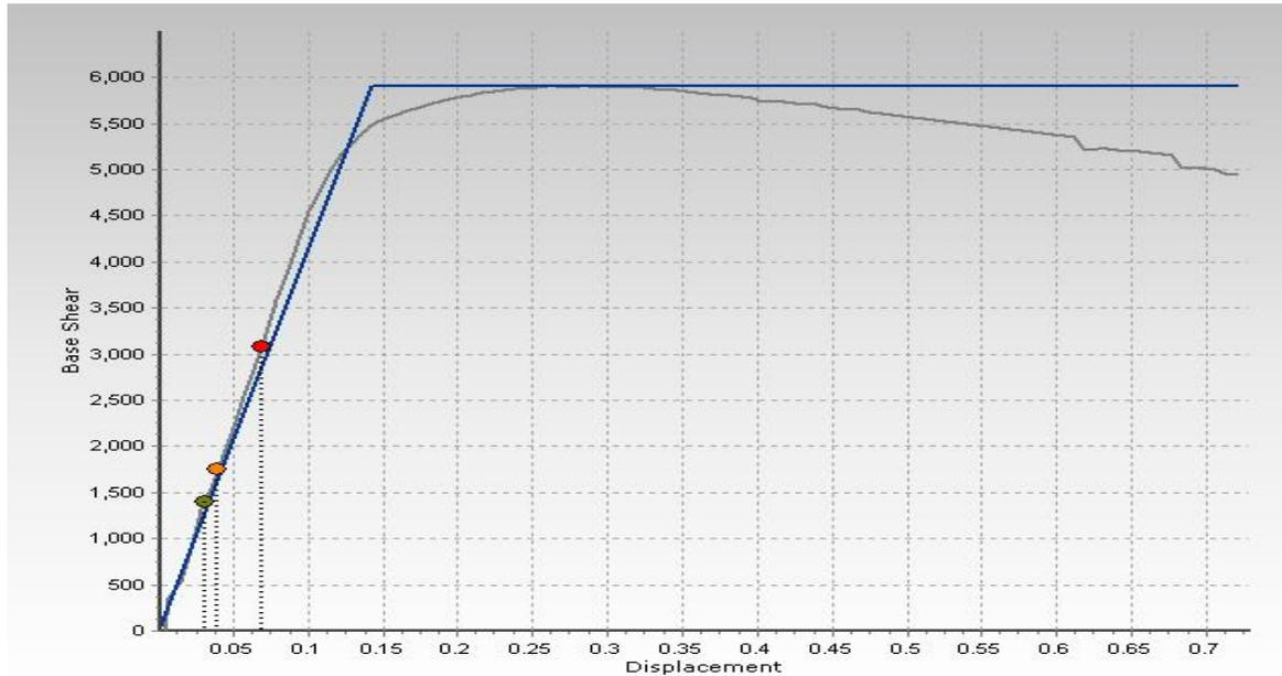
b) Figure 6.4 : Pushover –load –displacement curve for HSC-R MRF
