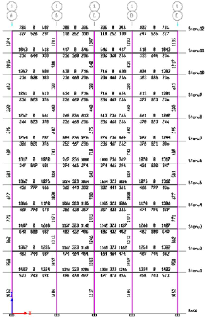
Figure B.4 HSC-SI frame design values ALONG SECTION 1-1
