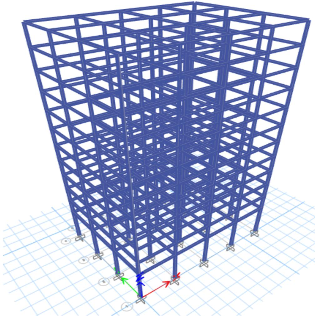
Figure 4.4 : Typical stiffness irregular MRF model -3D view
