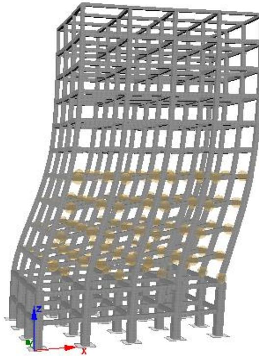
Figure 6.1: Deformed shape and plastic formation for NSC-R
