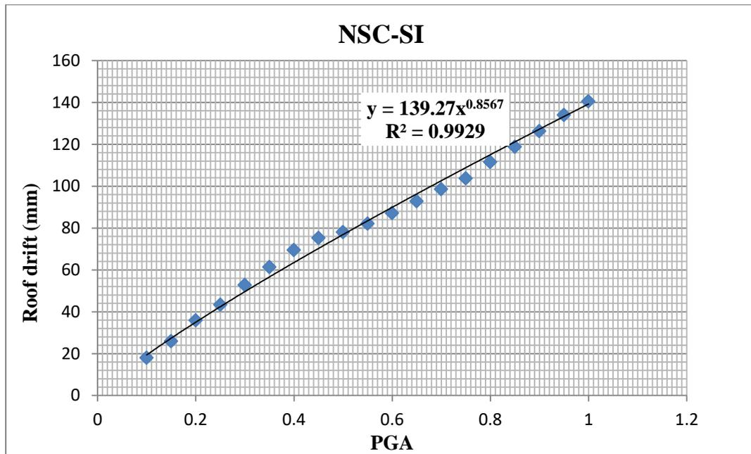
Figure 6.18: Probabilistic Seismic Demand Model of NSC-SI
