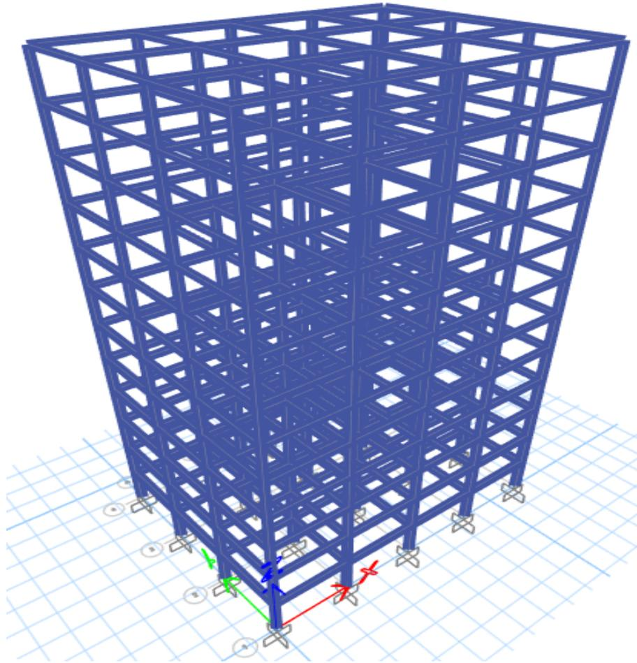
Figure 4.2: Typical stiffness regular MRF model -3D view
