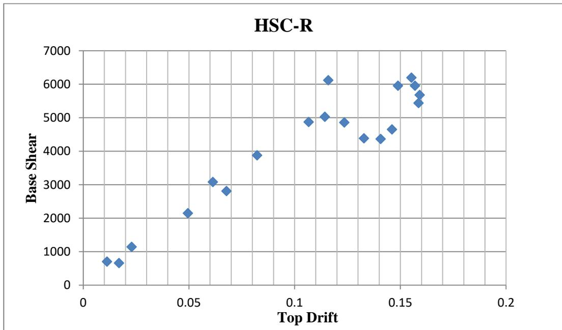
Figure 6.12: IDA capacity curve for HSC-R MRF
