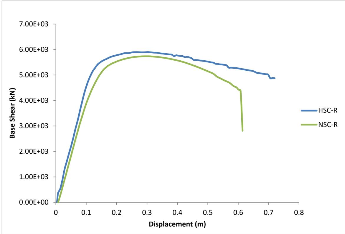
c) Figure 6.5 : Pushover result:- load –displacement curve for NSC-R and HSC -R on one graph.
