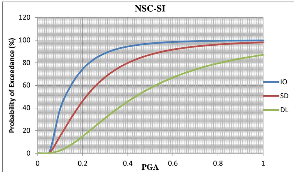
Figure E.3: Fragility curve of NSC-SI MRF
