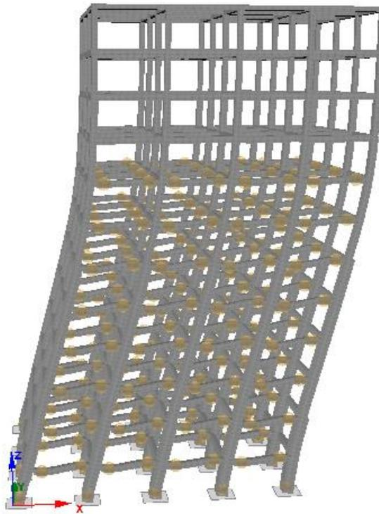
Figure 6.3: Deformed shape and plastic formation for HSC-R
