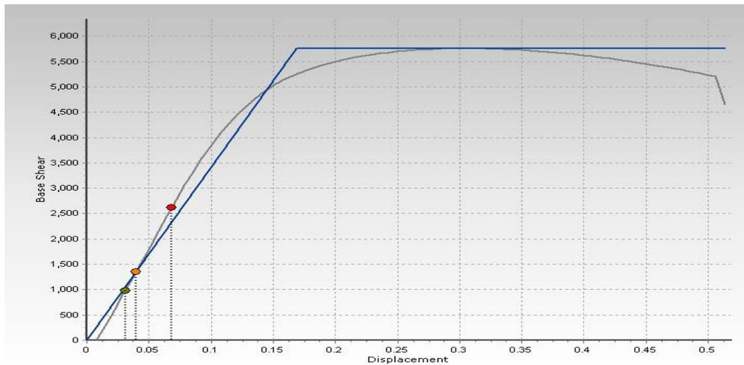
a) Figure 6.2 : Pushover –load –displacement curve for NSC-R MRF
