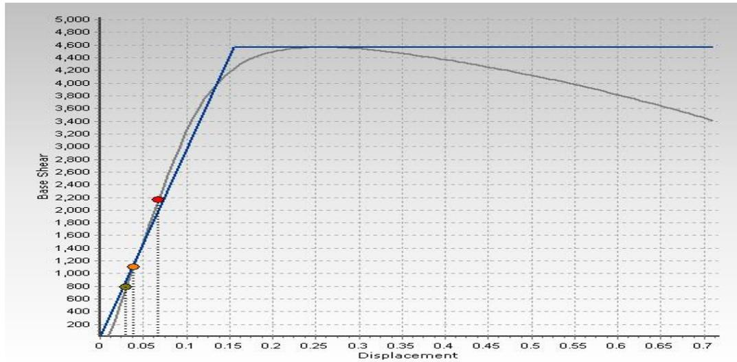
a) Figure 6.7 :Pushover –load –diplacement curve for NSC-SI MRF
