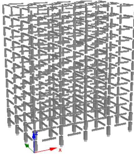
Figure C.1: 3D Seismostruct model for NSC-R MRF
