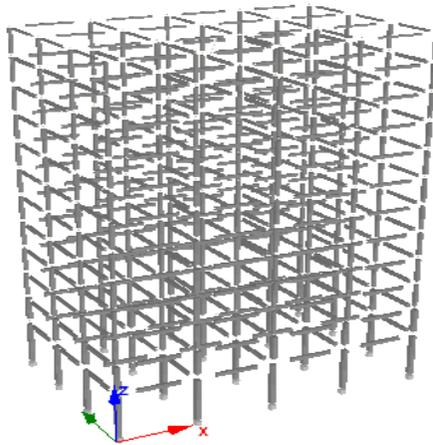
Figure C.4: 3D Seismostruct model for HSC-SI MRF
