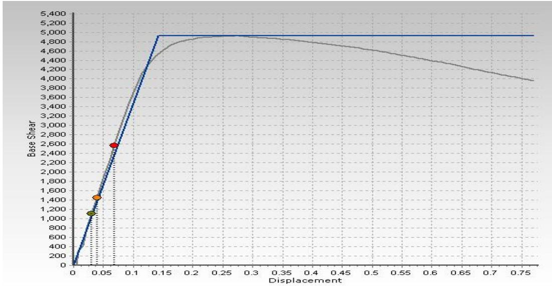
b) Figure 6.9: Pushover –load –displacement curve for HSC-SI MRF
