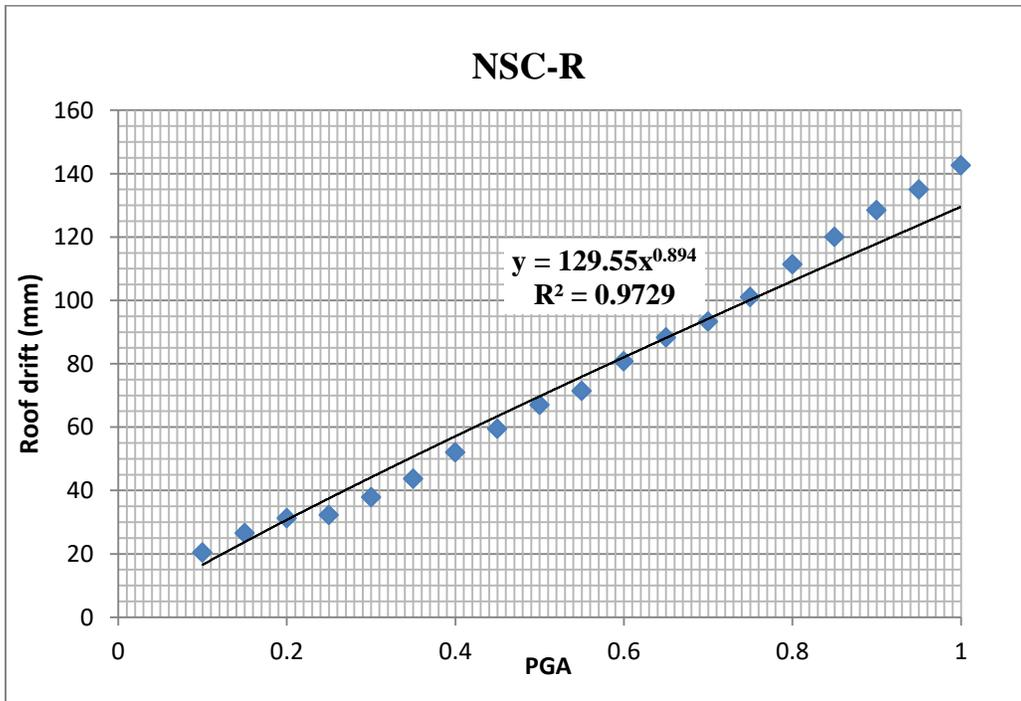
Figure 6.16: Probabilistic Seismic Demand Model of NSC-R
