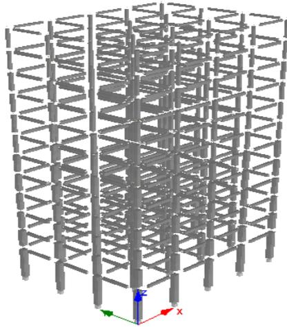
Figure C.3: 3D Seismostruct model for NSC-SI MRF
