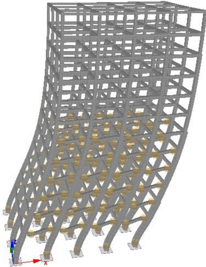
Figure 6.6: Deformed shape and plastic formation for NSC-SI
