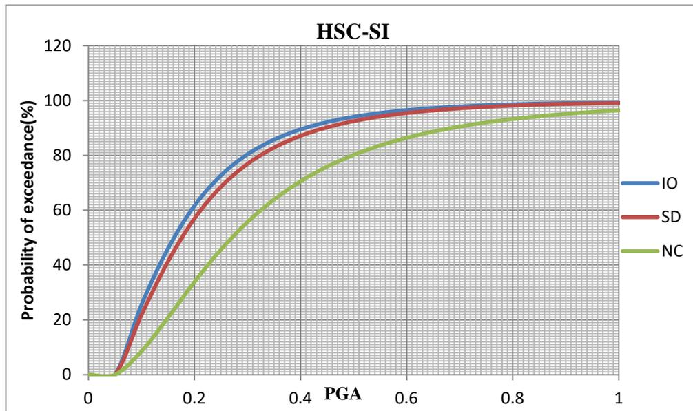
Figure E.4: Fragility curve of HSC-SI MRF
