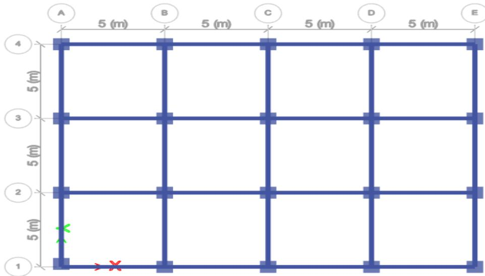
Figure 4.3 : Typical stiffness irregular MRF model -Plan view
