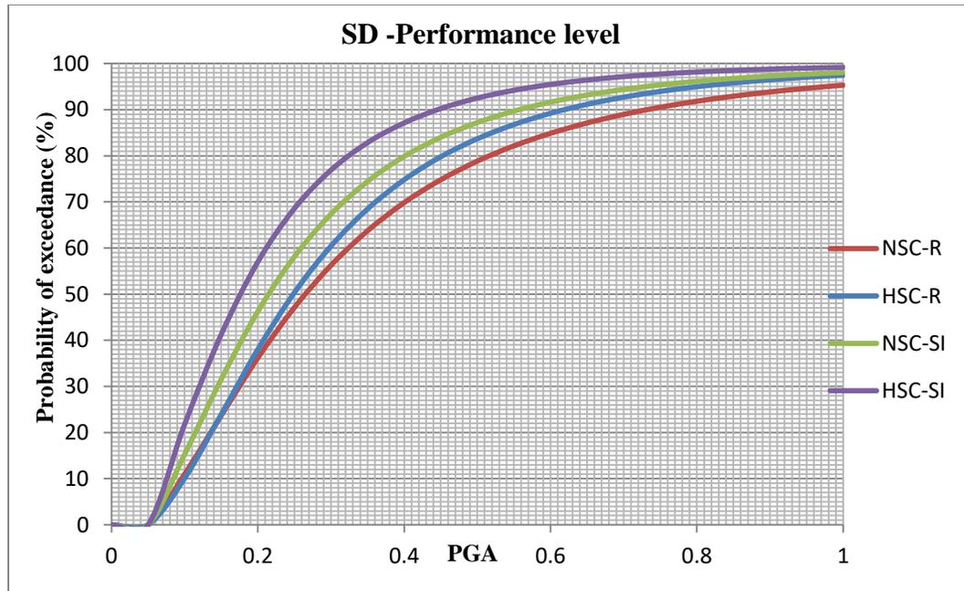
Figure 6.21: Fragility curve of both regular and stiffness irregular for SD Level
