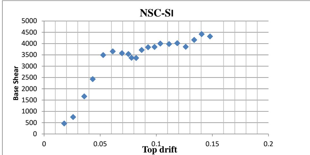
Figure 6.13: IDA capacity curve for NSC-SI MRF
