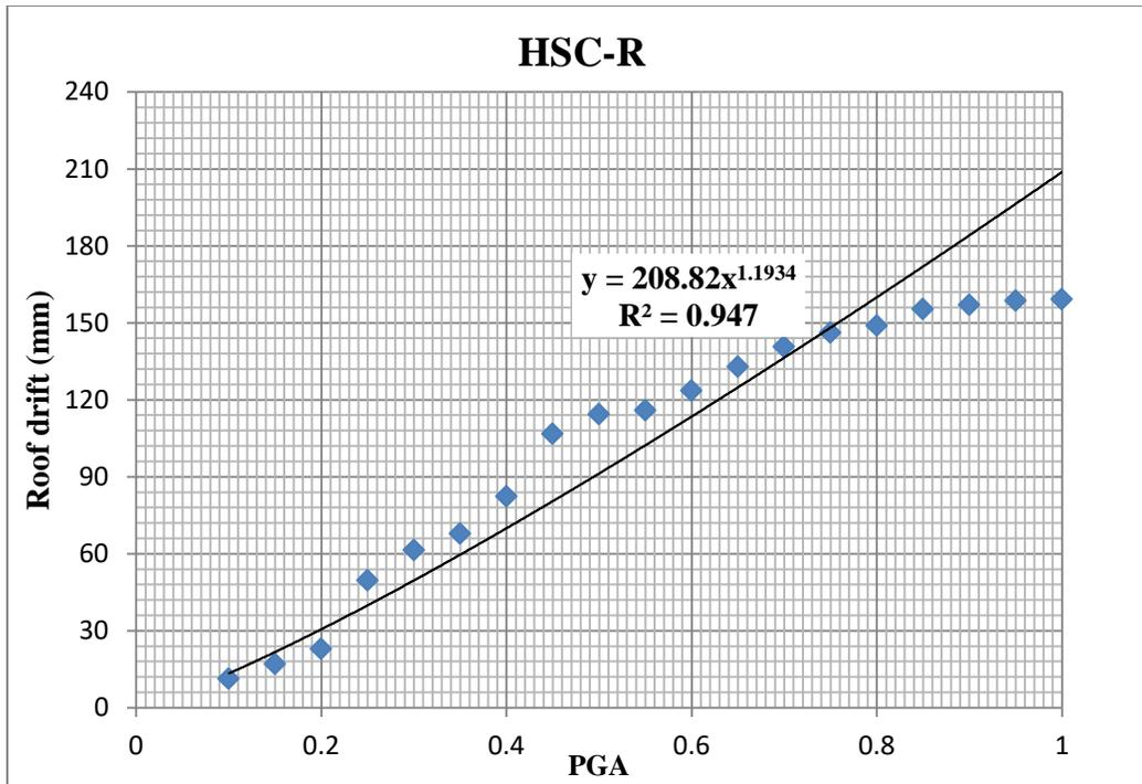
Figure 6.17: Probabilistic Seismic Demand Model of HSC-R
