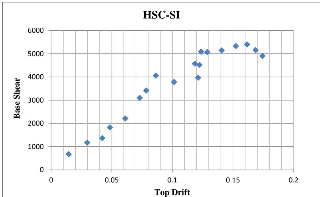
Figure 6.14: IDA capacity curve for HSC-SI MRF
