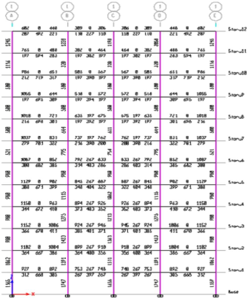
Figure B.1 NSC-R frame design values from ETABS v-18.1
