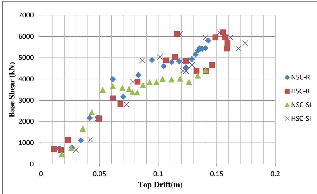
Figure 6.15: IDA capacity curve for all moment resisting (MRF)
