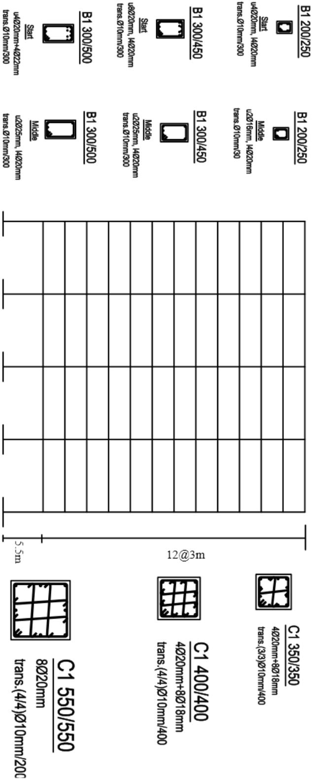
Figure 5.4: HSC-SI moment resisting frame (MRF) reinforcement detail
