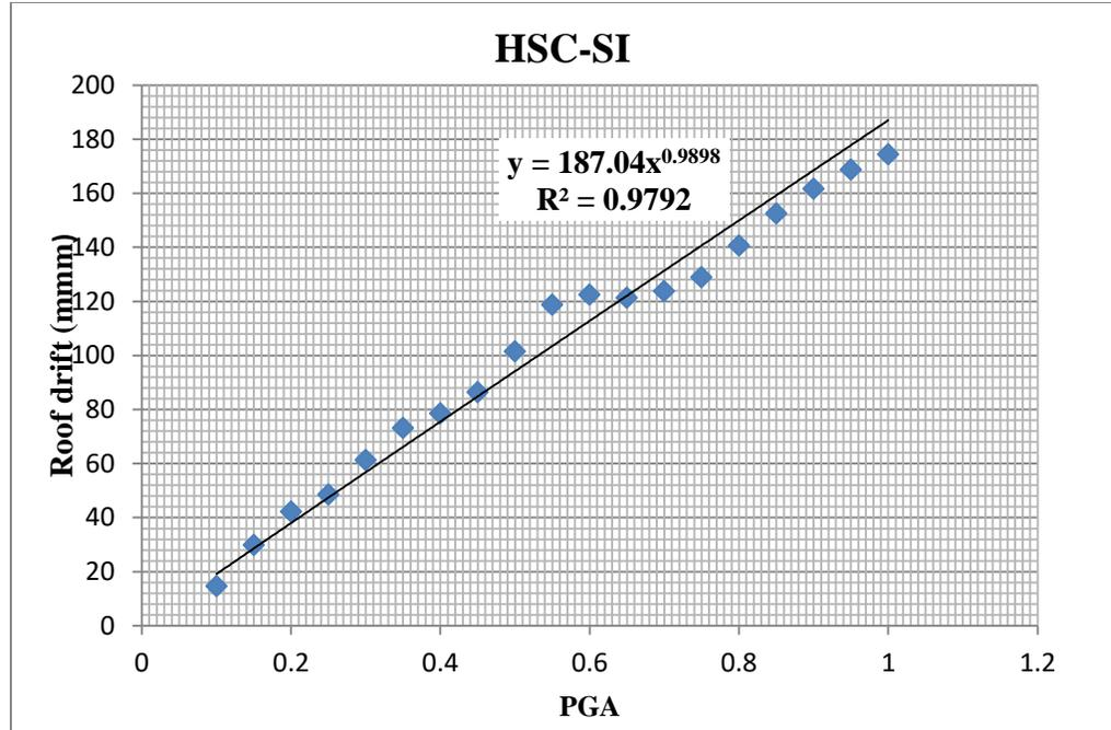
Figure: 6.19: Probabilistic Seismic Demand Model of HSC-SI
