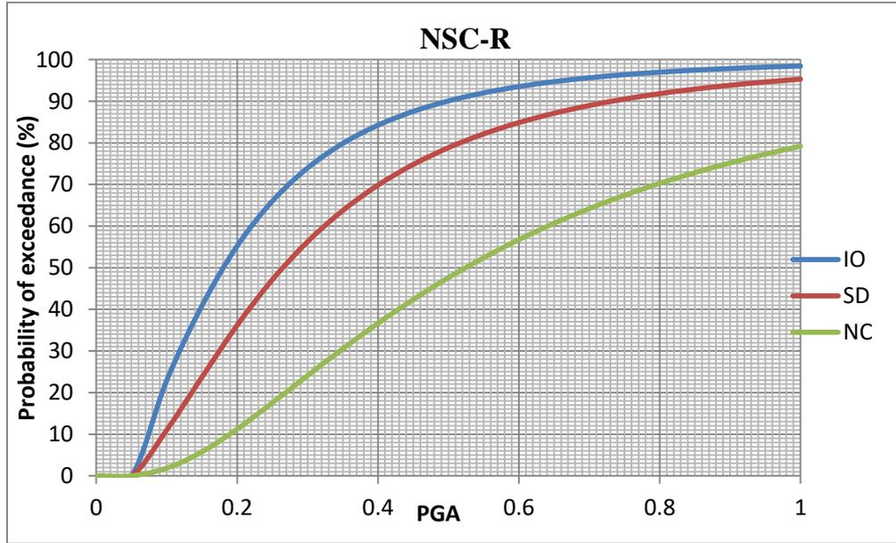
Figure E.1: Fragility curve of NSC-R MRF
