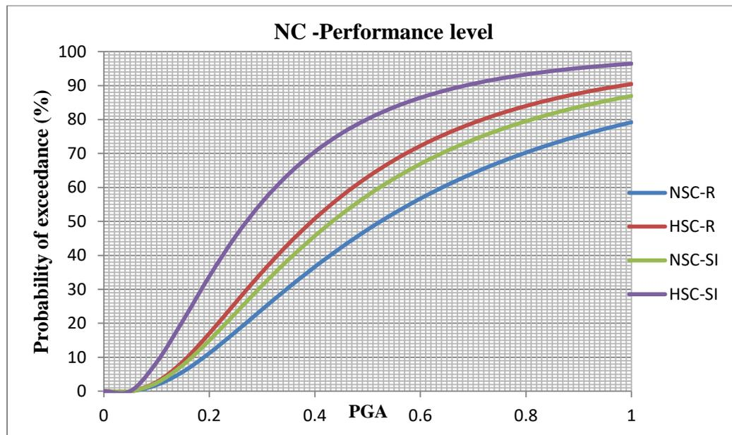
Figure 6.22: Fragility curve of both regular and stiffness irregular for NC Level
