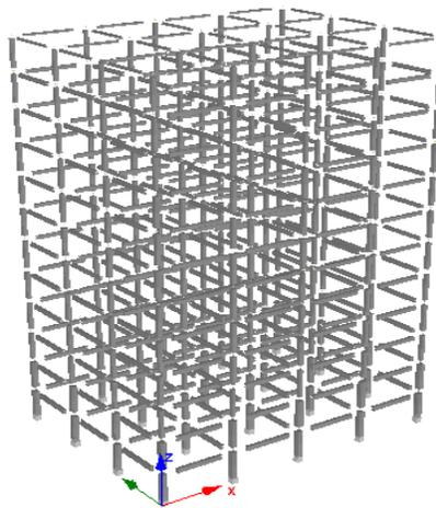
Figure C.2: 3D Seismostruct model for HSC-R MRF
