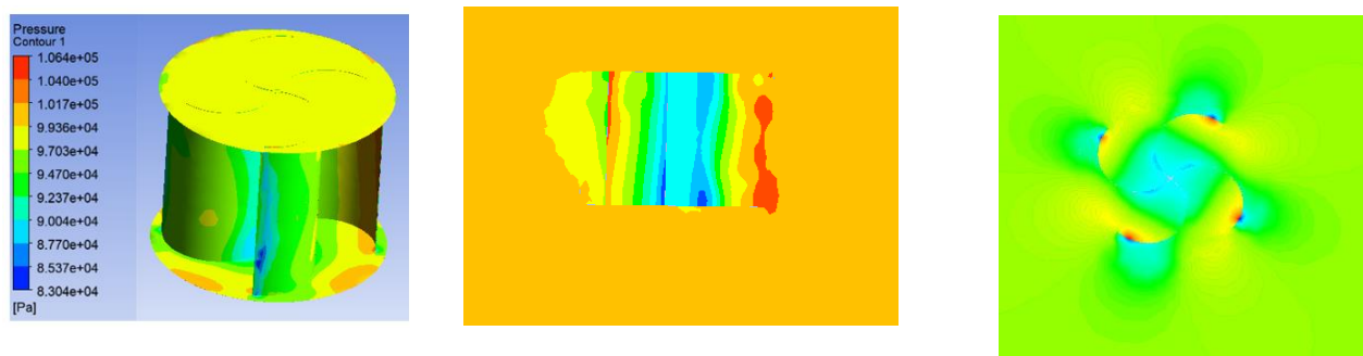
Figure 5.3 Pressure distribution of Savonius rotor without fin
