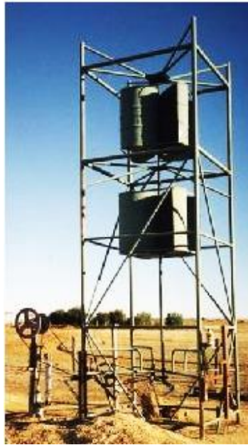
Figure 2. 1 Savonius wind turbine for the application of water pumping (Argaw, Foster, and Ellis, 2003)
