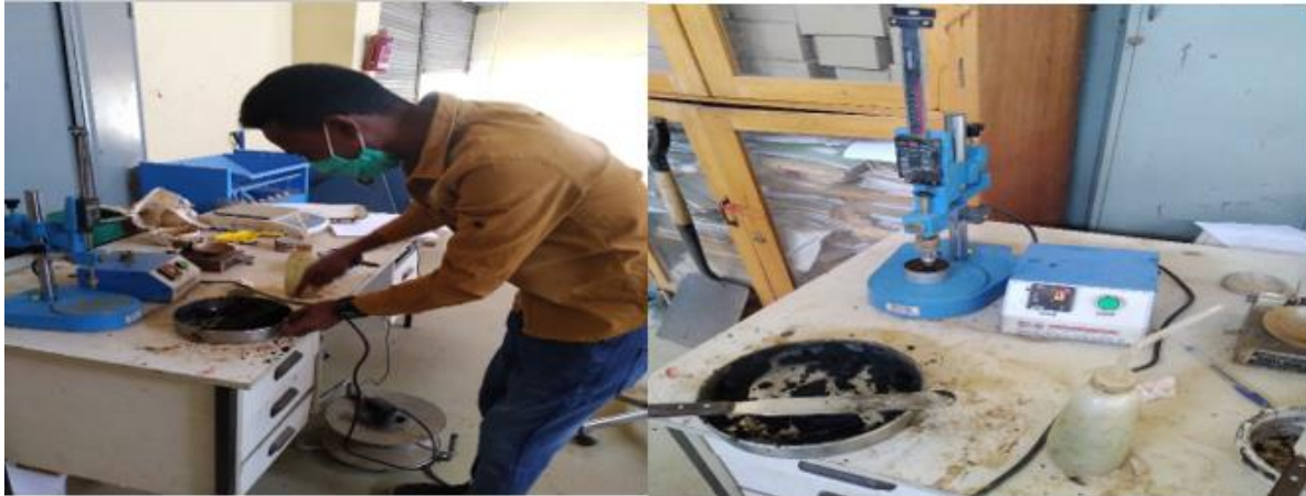
Soaking the BA and SSD and Ready the sample for liquid limit test (Source Dejene Dereje,2014).
