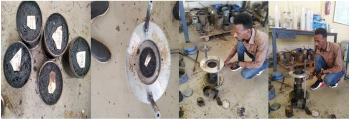
Compacted hot mix asphalt concrete specimens cool down and extracted (removed in mold) (Source Dejene Dereje,2014)
