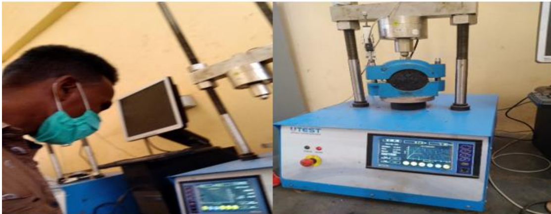
Recording the Marshall Test results stability and flow of specimens (Source Dejene Dereje,2014).
