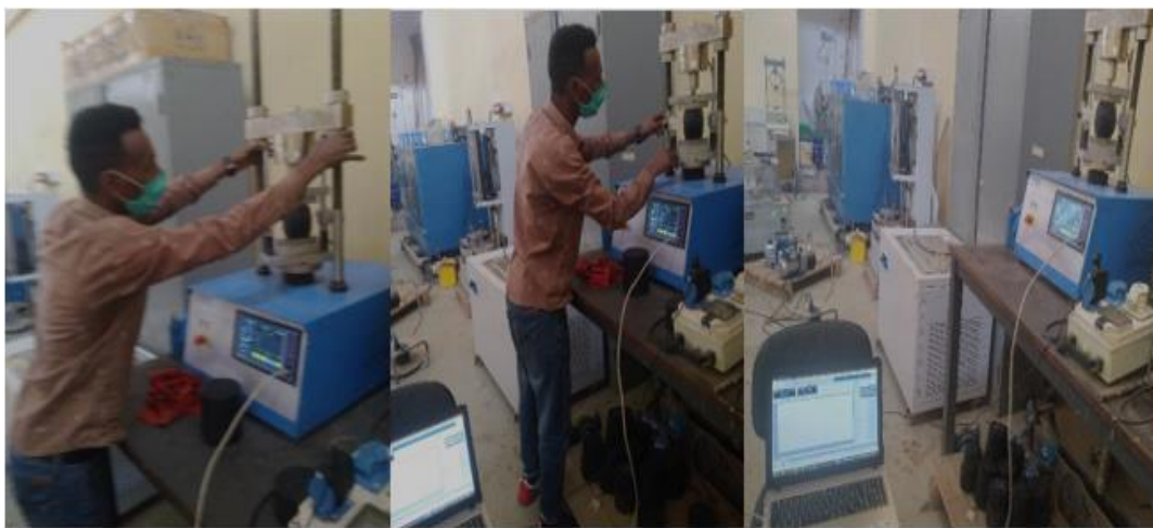
Recording result of conditioned and unconditioned the Marshall Test results of specimens for determine the value of TSR (Source Dejene Dereje,2014).
