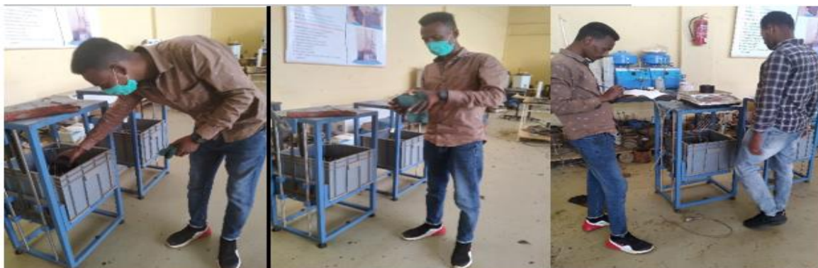
Making dry specimen by cloth after weight in water and also weighting specimen after dry (Source, Abebe Tadie,2014).
