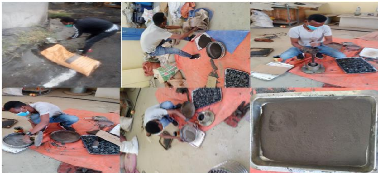
Figure 3.2. The process of cleaning /crushing, milling and sieving of steel slag dust and bagasse ash fillers from the source to in the laboratory (Source, Dejene Dereje,2014).
