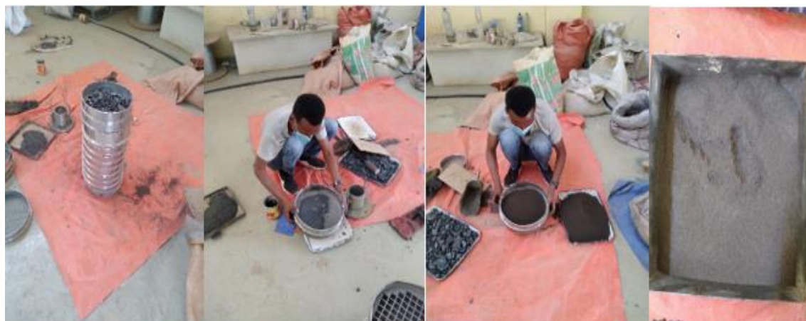
Sieve arrangement by size and sieve the aggregates by different sieve number (Source Dejene Dereje,2014)
