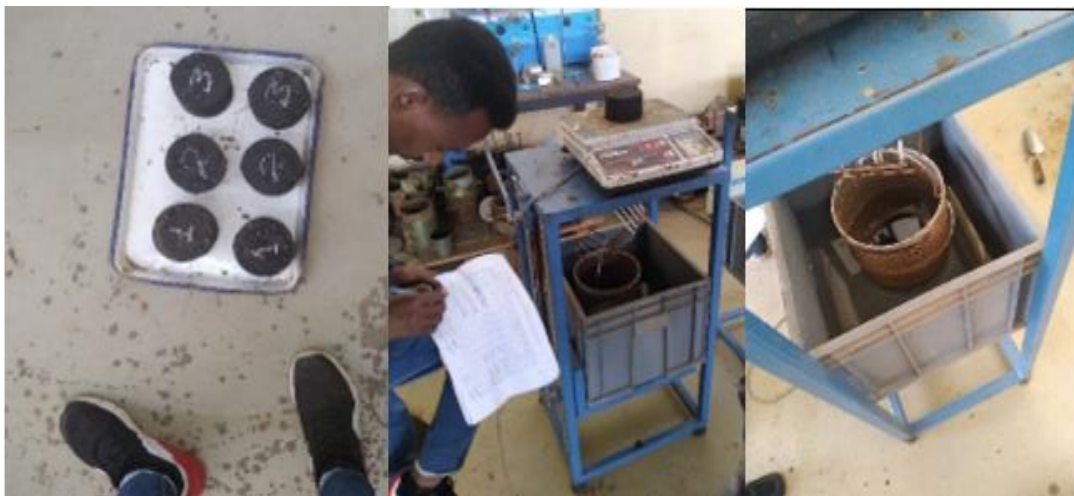
Weighting the hot mix asphalt specimen after air dry and in water (Source Dejene Dereje,2014).
