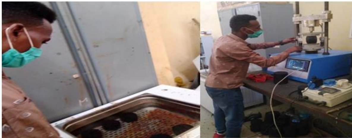
Figure 3.5. Removal of the specimen from the immersed water bath and measuring of Stability and flow by using Marshall Tester machine (Source, Dejenie Dereje,2014).
