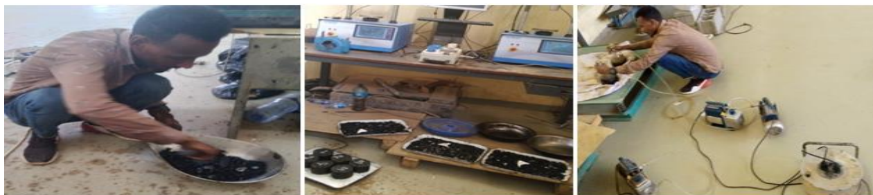
Figure 3.6. Mixing and cooling down of samples for specific gravity (Source. Dejenie Dereje,2014).
