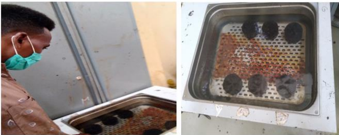
Sink the specimen in water bath at 45°C for measuring stability and flow (Source Dejene Dereje,2014).
