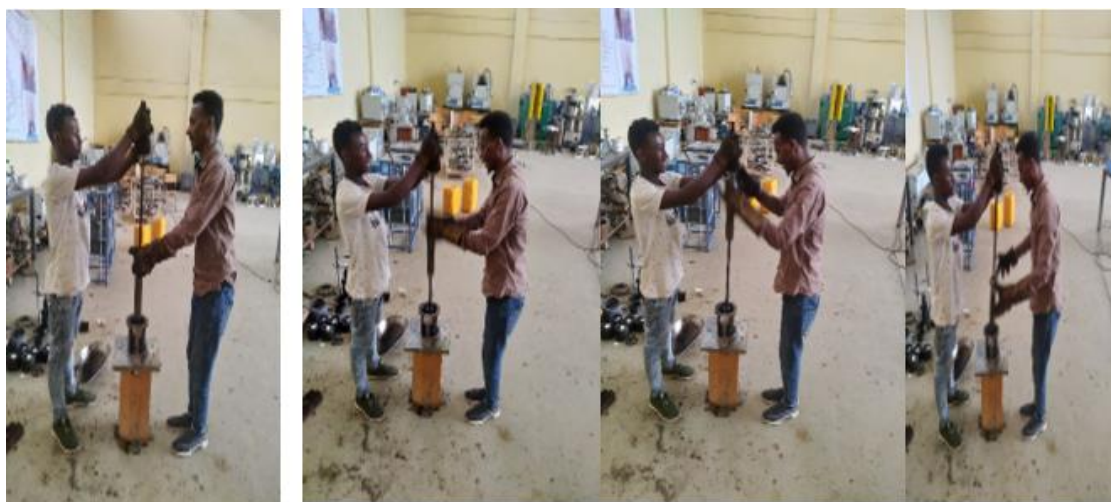
Compacted mixed materials by using compactor machine manually (Source Dejene Dereje,2014).
