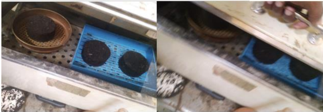
Sink the specimen in water bath at 45°C and in cool water bath for measuring TSR at optimum replacement of non-conventional (Source Dejene Dereje,2014).
