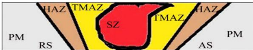
Figure 2. 6 Different characteristic zones of FSW/UFSW (Threadgill 1997)
