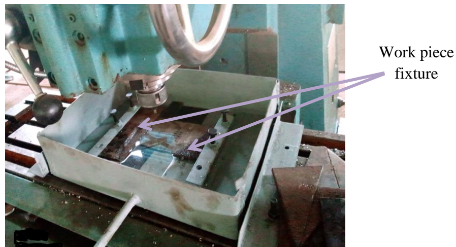
Figure 3. 7 Container and work piece holder/fixture
