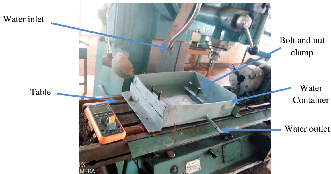
Figure 3. 2 view of sample prior to welding and holding fixture
