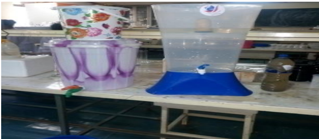
Figure 3 Modified sand with ceramic candle filter
