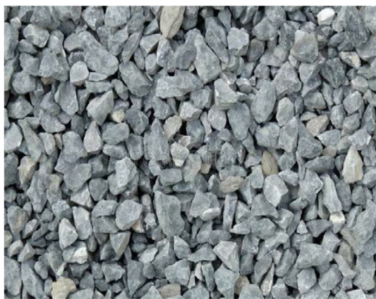
Figure 3. Crushed stone aggregate.
