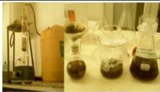
Figure 6. The soxhlet (right) and maceration (left) techniques of extraction used for the study.
