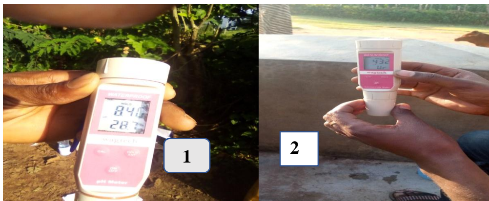
Figure 5; Measuring (1) PH and temperature (2) conductivity on site.
