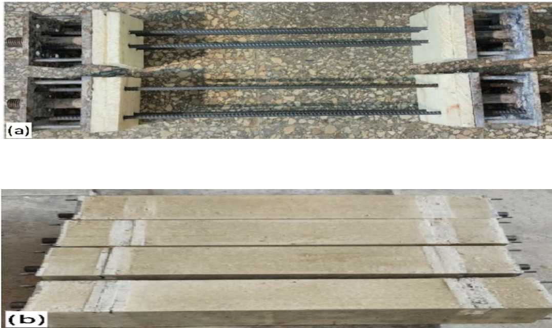
Figure 10: Tension prismatic specimens: (a) Reinforcement skeletons before placement into the moulds; (b) Specimens brought out of the moulds (Gribniak et al. , 2020).
