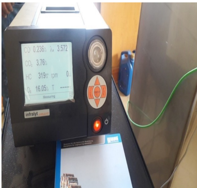
a) Emission analysis of pure diesel
