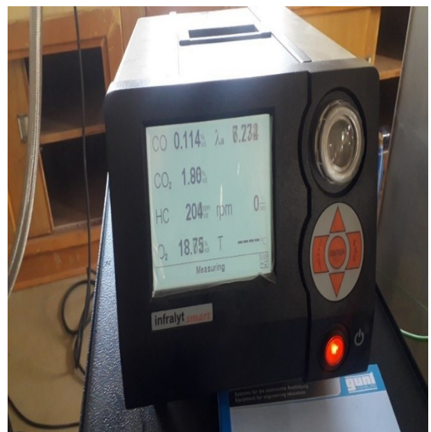
b) Emission analysis of biodiesel- diesel B 5 blend
