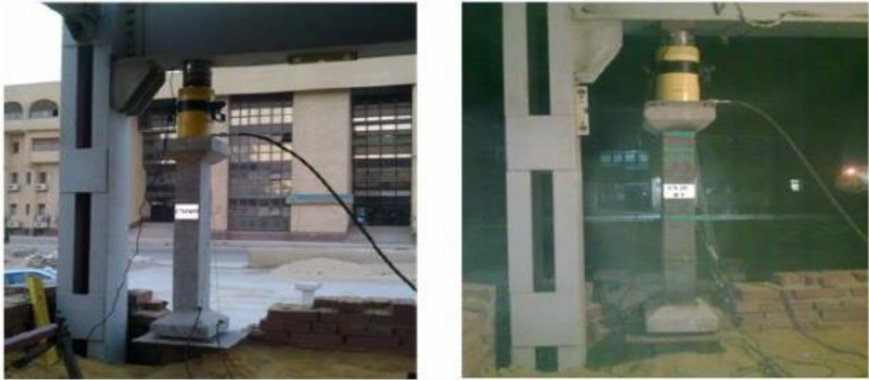
Figure 4.2 Experimental setup for the test used for steel jacketing (Ezz-eldeen, 2018)
