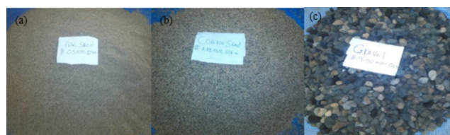
Fig. 3 Sand materials: - fine sand (a); coarse sand (b) and gravel (c) after sieve analysis in the laboratory
