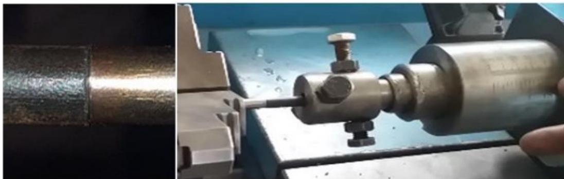
Fig. 3.6: Stationary arrangements of newly CDFW set up in lathe machine
