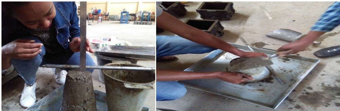
Photo:- workability test
