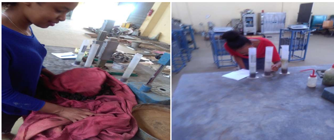
Photo:-specific gravity for coarse aggregate and silt content test for fine aggregate
