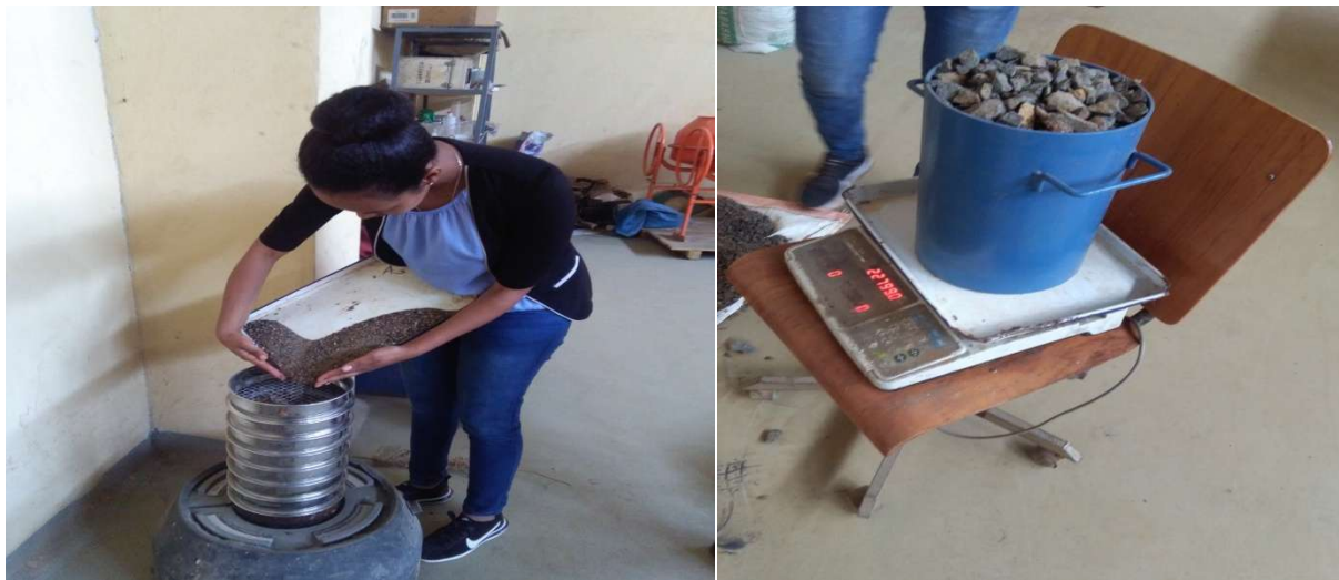
Photo:-Siveanalysisi for fine aggregate and unit weight for coarse aggregate
