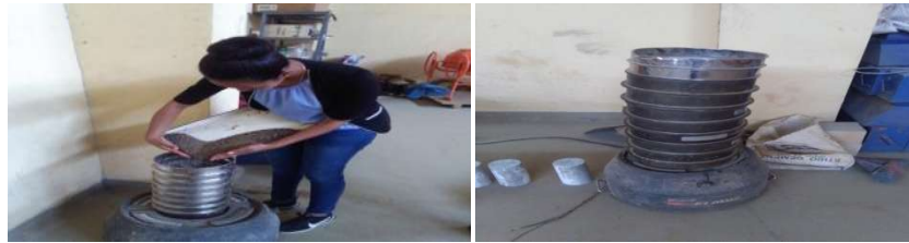
Figure 3.5- Sieve Size of Fine Aggregate and Coarse Aggregate
