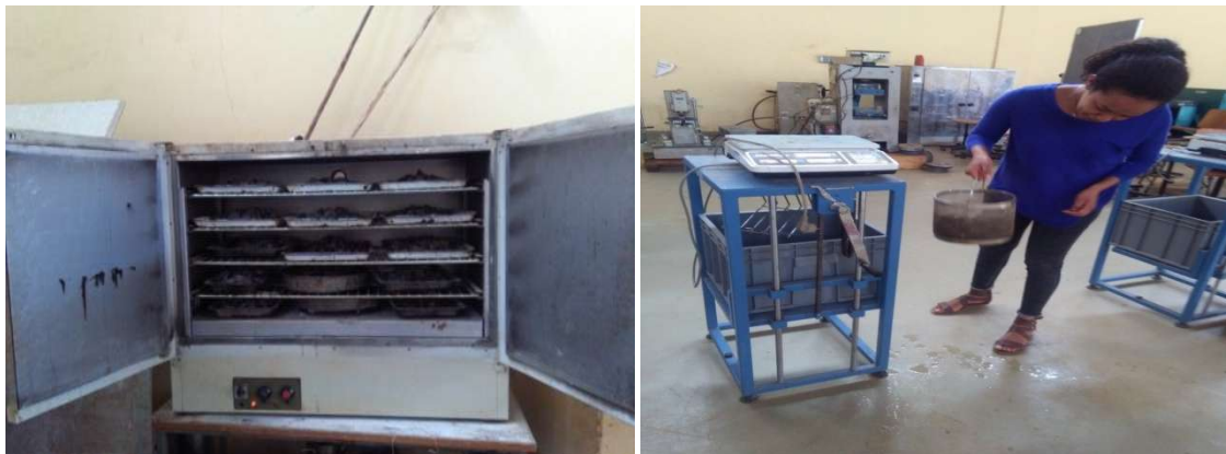
Photo:-Specific Gravity for coarse aggregate
