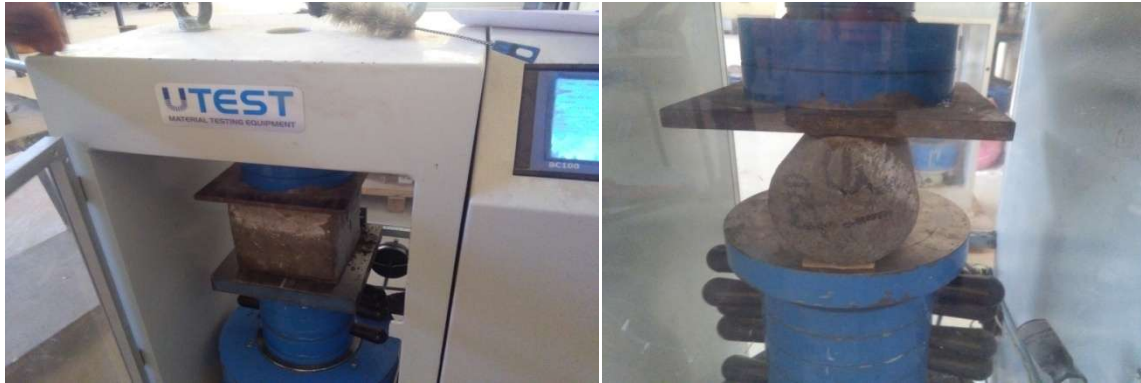
Photo:- compressive strength and split tensile strength test
