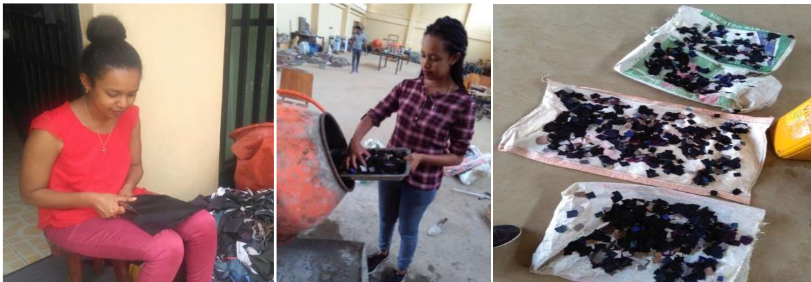
a. Cutting Textile fiber b. Mixing the textile piece c. drain washed Textile cut sample
