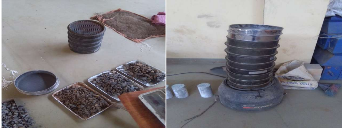
Photo:-sive analysis for coarse aggregate
