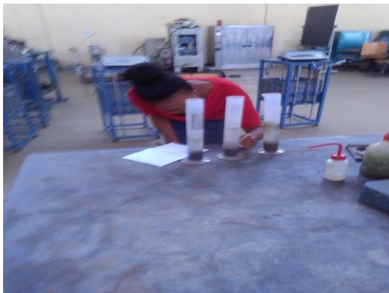
Figure 3.3- Silt Content of Sand
