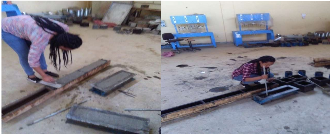
Photo:compacting and finishing mold concrete
