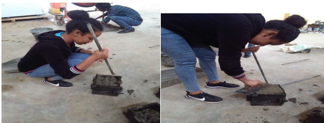
Photo:compacting and finishing mold concrete
