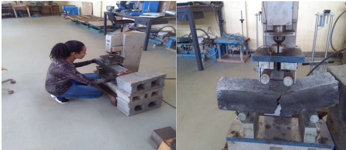
Photo:- Flexural strength test
