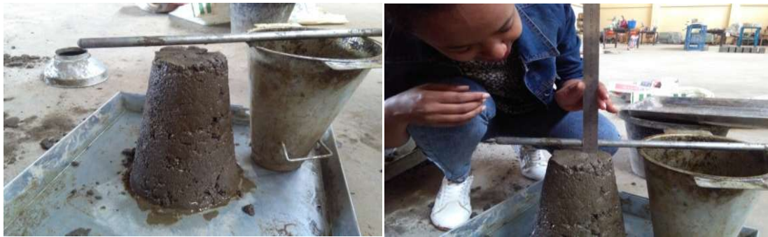
Figure 3.8- Workability Test Samples
