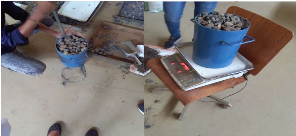
Figure3.4 :- Unit weight for coarse aggregate
