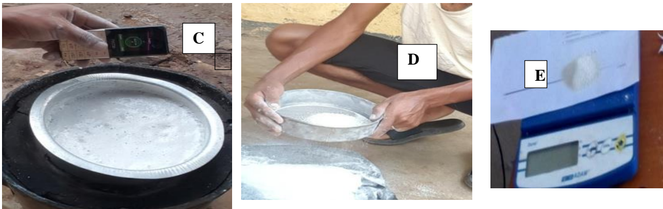
Fig; A crushing of lime, B & E measuring of soil and lime, C&D 5minute reactivity test on lime and finest test of lime respectively
