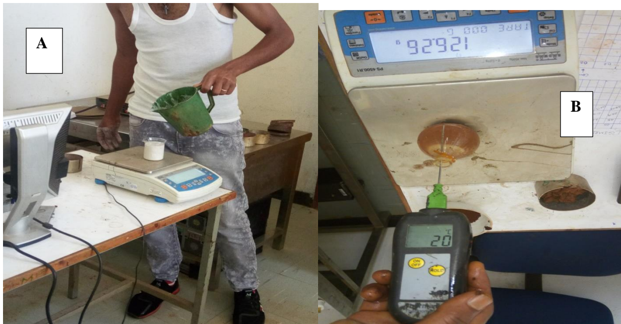
Figure; A Density test of lime and B Specific gravity test of soil
