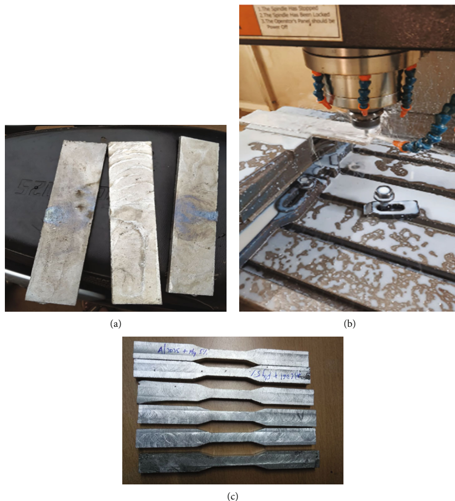
FIGURE 4: Work pieces. (a) Casting work pieces. (b) Process of machining. (c) Final specimens of different composition.
