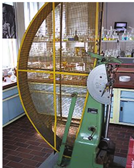
FIGURE 11: Machinery used for Impact test.
