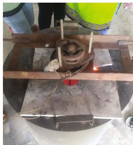
FIGURE 2: Stir casting setup.
