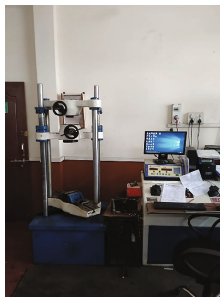
FIGURE 5: Setup for computing UTS.
