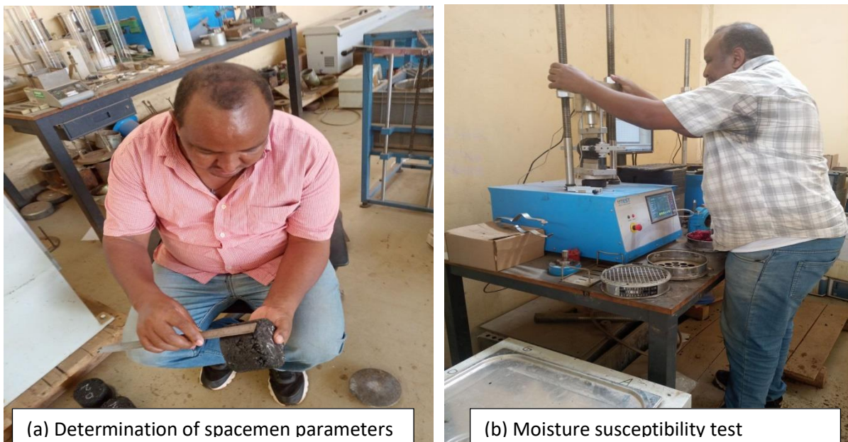
Figure 5.8 (a) Determination of specimen parameters (b) Moisture susceptibility test (captured by Bimiyam B.)
