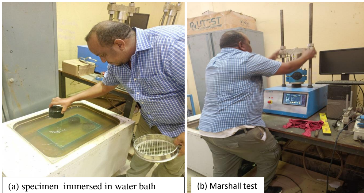
Figure 3.5 (a) specimen immersed in water bath, (b) Marshall test captured by Biniyam B.
