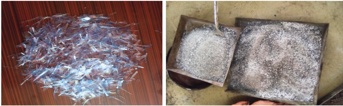
FIGURE 2: Waste marble and plastic strips prepared for tests.
