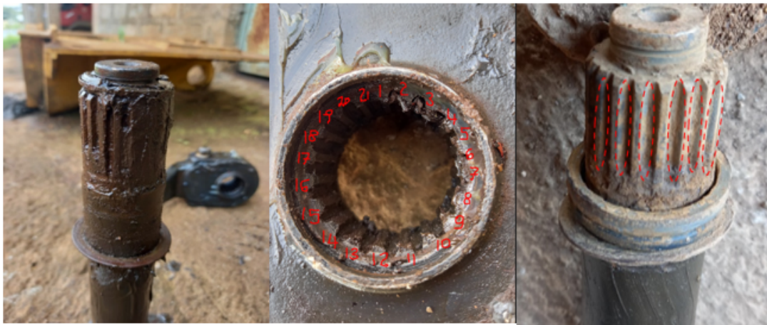
Figure 1.10: Failed shaft and hub with surface wear damage due to minor pitting
