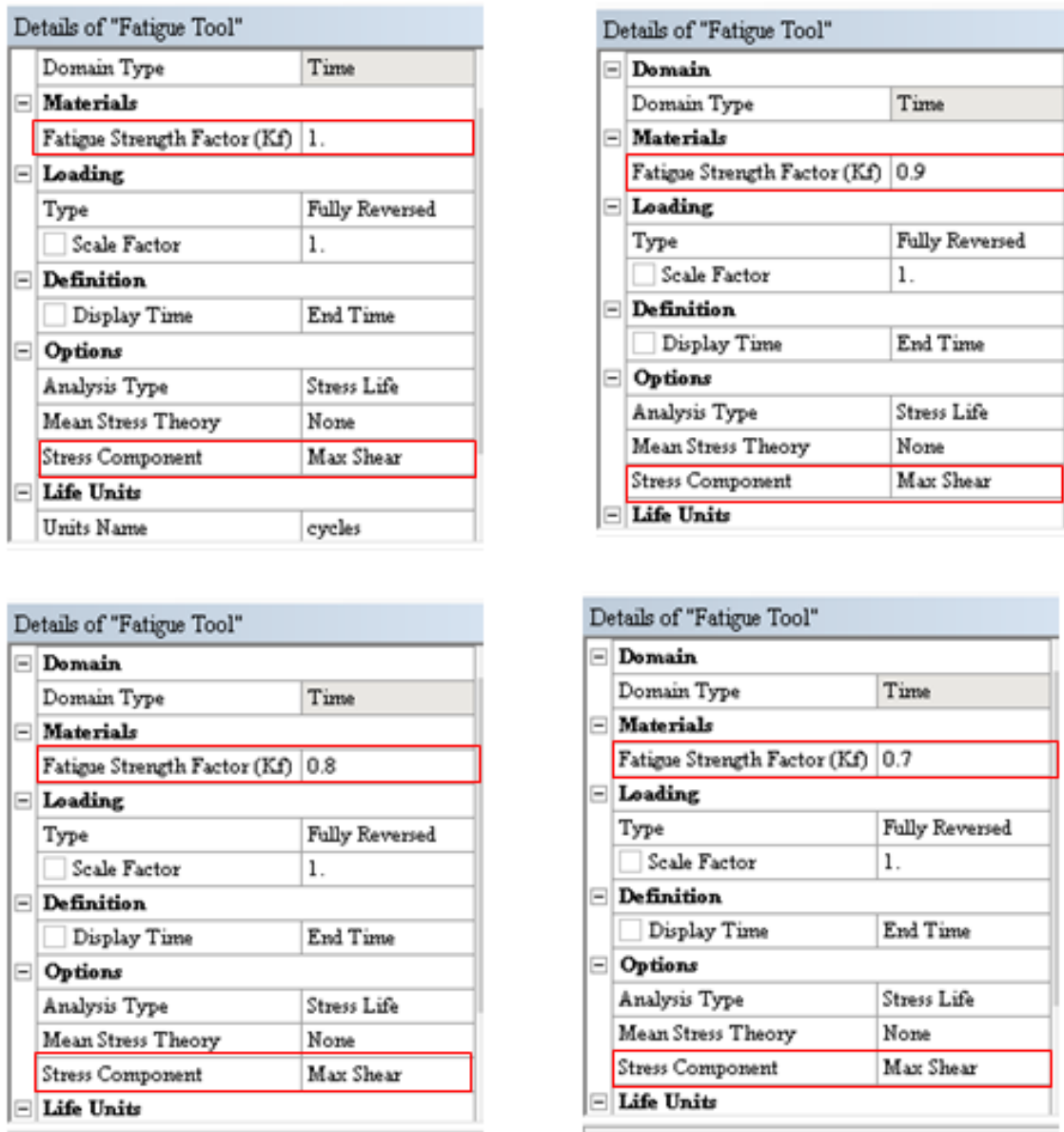
Figure 5.7: Maximum shear stress for fully reverse loading conditions on different fatigue strength factors
