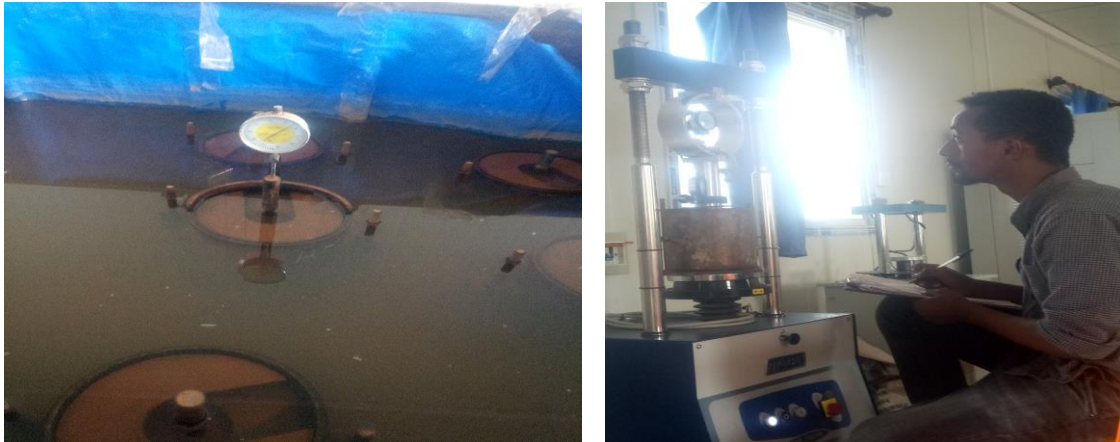
Figure 3. 17: Recording swell and penetration data
