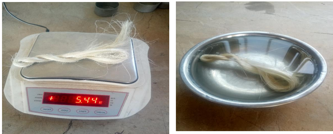
Figure 3. 13: Measuring and soaking the sample to determine absorption rate
