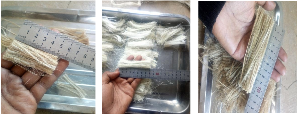
Figure 3. 15: Sisal fiber chopped in 5cm, 8cm and 11cm
