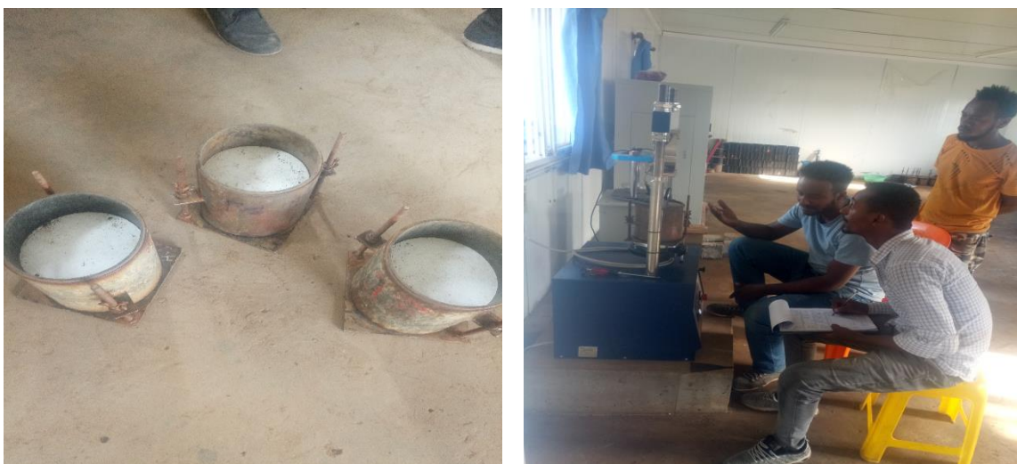
Figure 3. 11: Sample prepared for soaking and penetration reading
