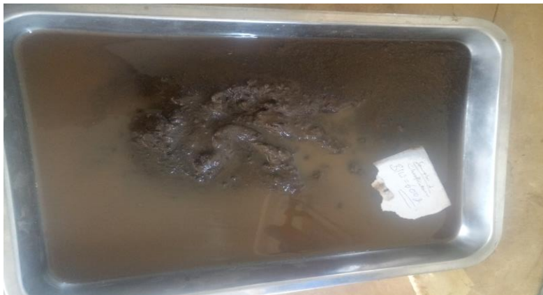
Figure 3. 7: Soil sample soaked for wet sieve analysis
