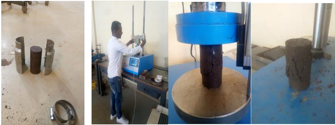
Figure 3. 12: Unconfined compression test
