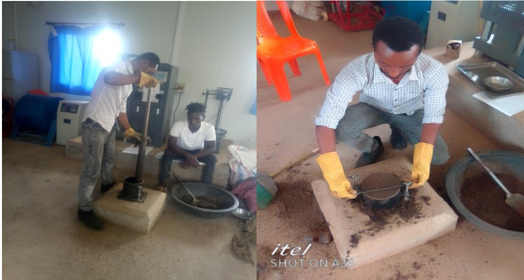
Figure 3. 10: Compacting and trimming soil sample
