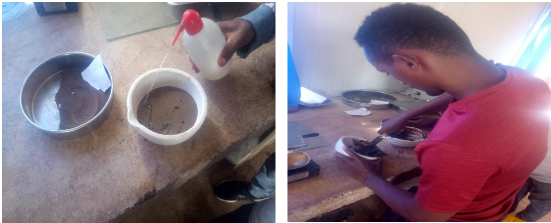
Figure 3. 8: Soaking and mixing soil sample respectively for LL and PL
