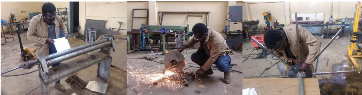
Figure 3.3 Manufacturing process of spiral pump prototype in Mechanical engineering laboratory
