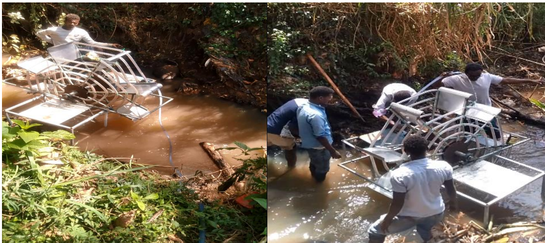
Figure 1.2 Spiral pump testing on Awetu River
