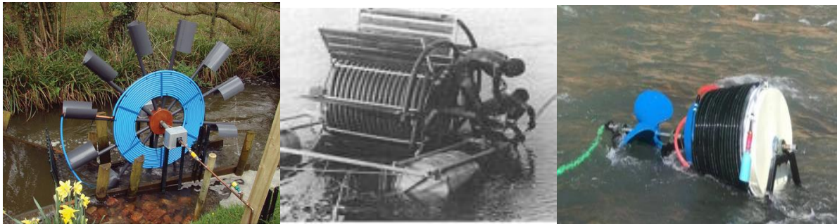
Figure 2.2 From Right to left; Spiral pump, Coil pump, and Conical Helix pump [23]
