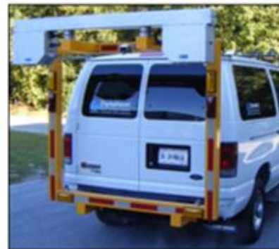
Figure 2.12. a) Automatic Condition Survey and Falling Weight Deflectometer b) Dynatest Multifunction Vehicle [24].
