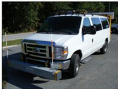
Figure 2.12. a) Automatic Condition Survey and Falling Weight Deflectometer b) Dynatest Multifunction Vehicle [24].
