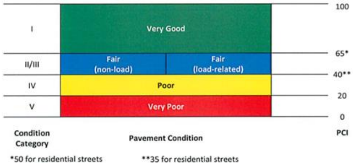
Figure 2.5. Pavement Condition Categories [29].
