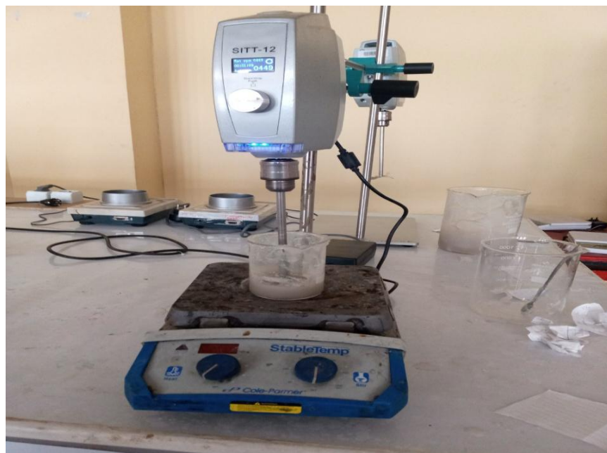
Figure 24:- mechanical stirrer with combination of stove
