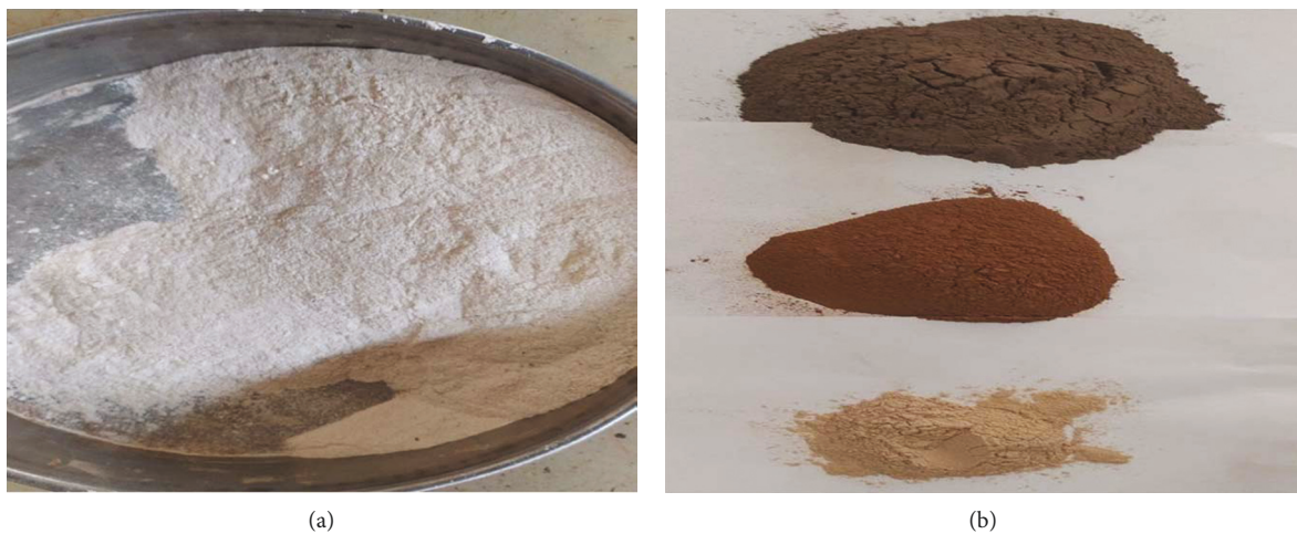
FIGURE 2: Prepared sample: (a) powdered glass and (b) soil and stabilizers.
