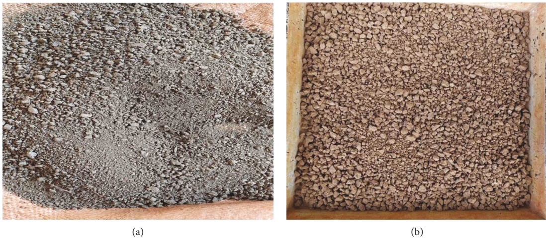
FIGURE 1: Soil sample: (a) air dried and (b) kilned/burned.
