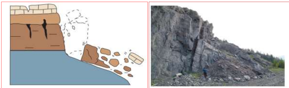
Figure 2.3 Schematic of a topple failure in Canada (Source: (Highland and Bobrowsky, 2008)).
