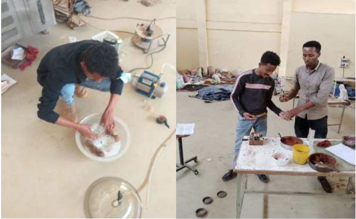
Figure D3. Photos taken during Specific gravity and Atterberg Limits determination.
