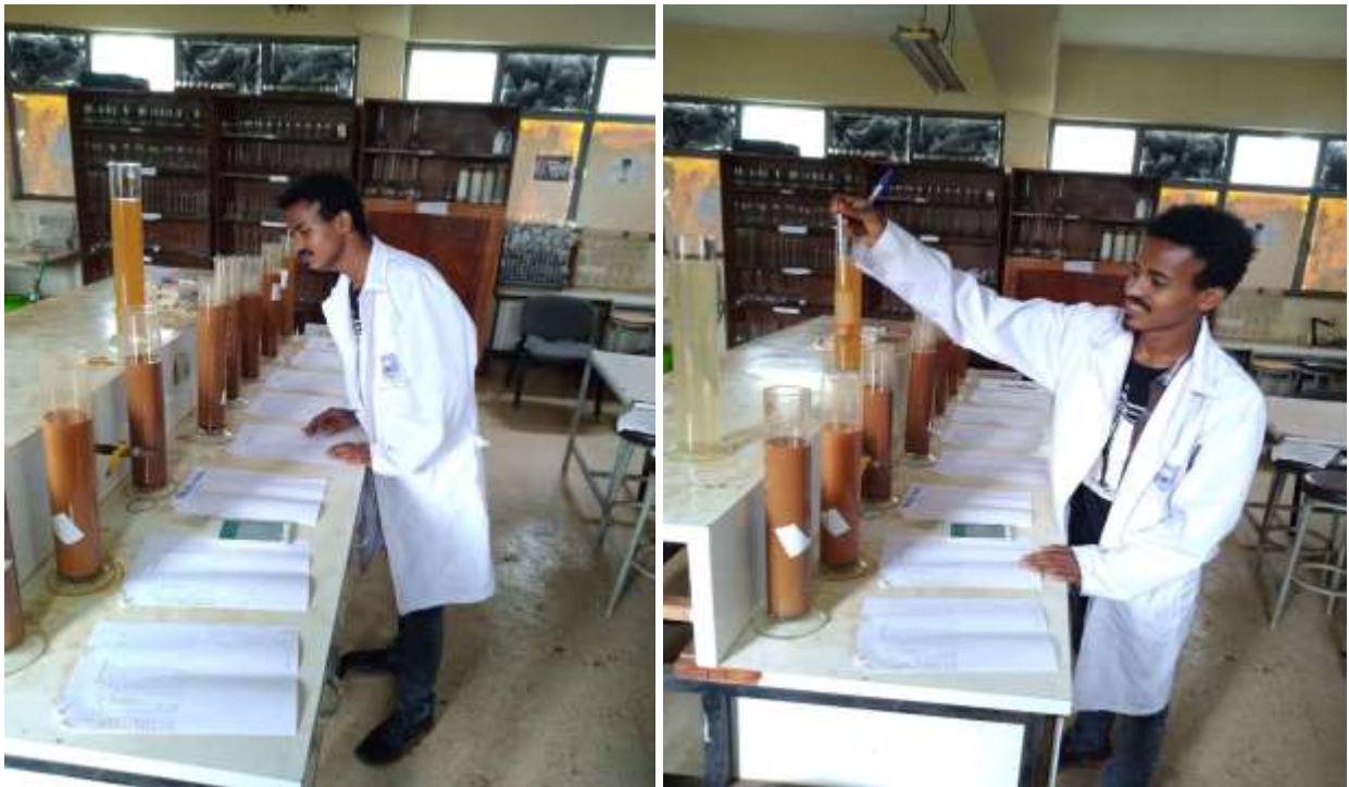
Figure D4. Photo taken during Hydrometer analysis testing.
