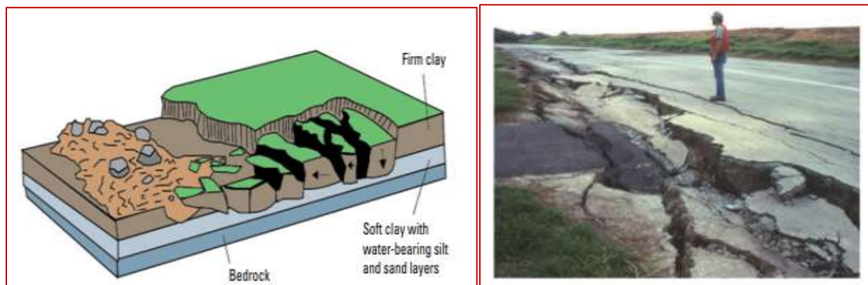
Figure 2.5 Schematic of Spread Failures and Due to the 1989 Loma Prieta, California, USA earthquake, lateral spread damage to a roadway ( Source: (Highland and Bobrowsky, 2008))
