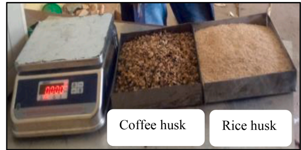
Fig. 10. Coffee and rice husk biomass samples for predicting the porosity and void ratio.
