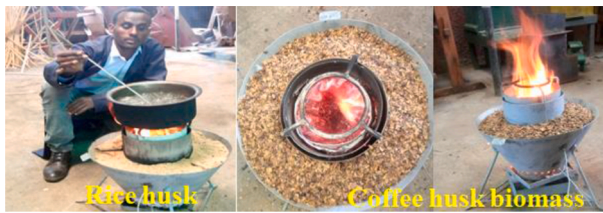
Fig. 17. The WBT flame photo's using coffee husk and rice husk biomass.
