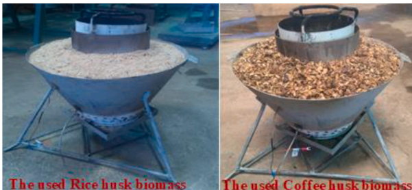
Fig. 8. The WBT experiment set up for using rice husk and coffee husk biomass.
