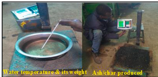
Fig. 18. Water temperature and ash or char produced during the test.
