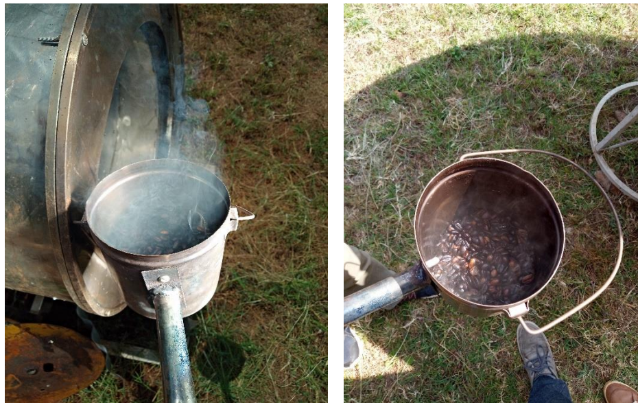
Figure 3. 12 roasting coffee using scheffler reflector
