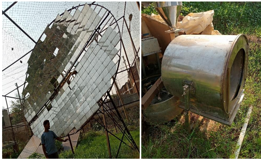
Fig. (a)Scheffler dish installed at JUCAVM (b) receiver (absorber)
