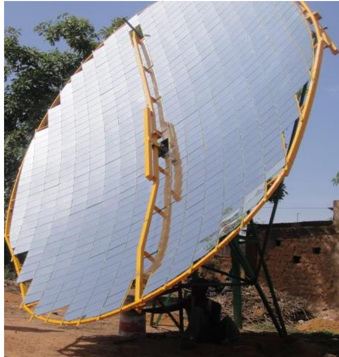
Figure 2. 2 a Scheffler dish [3]
