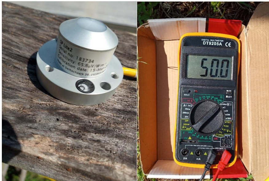
Fig. Pyranometer and its digital multi meter
