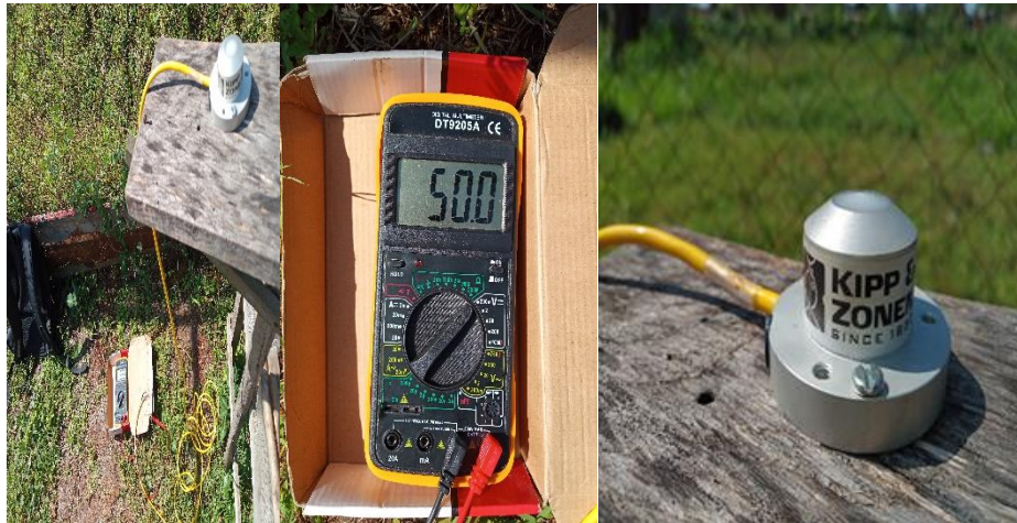
Figure 3. 14 pyranometer with its multi meter
