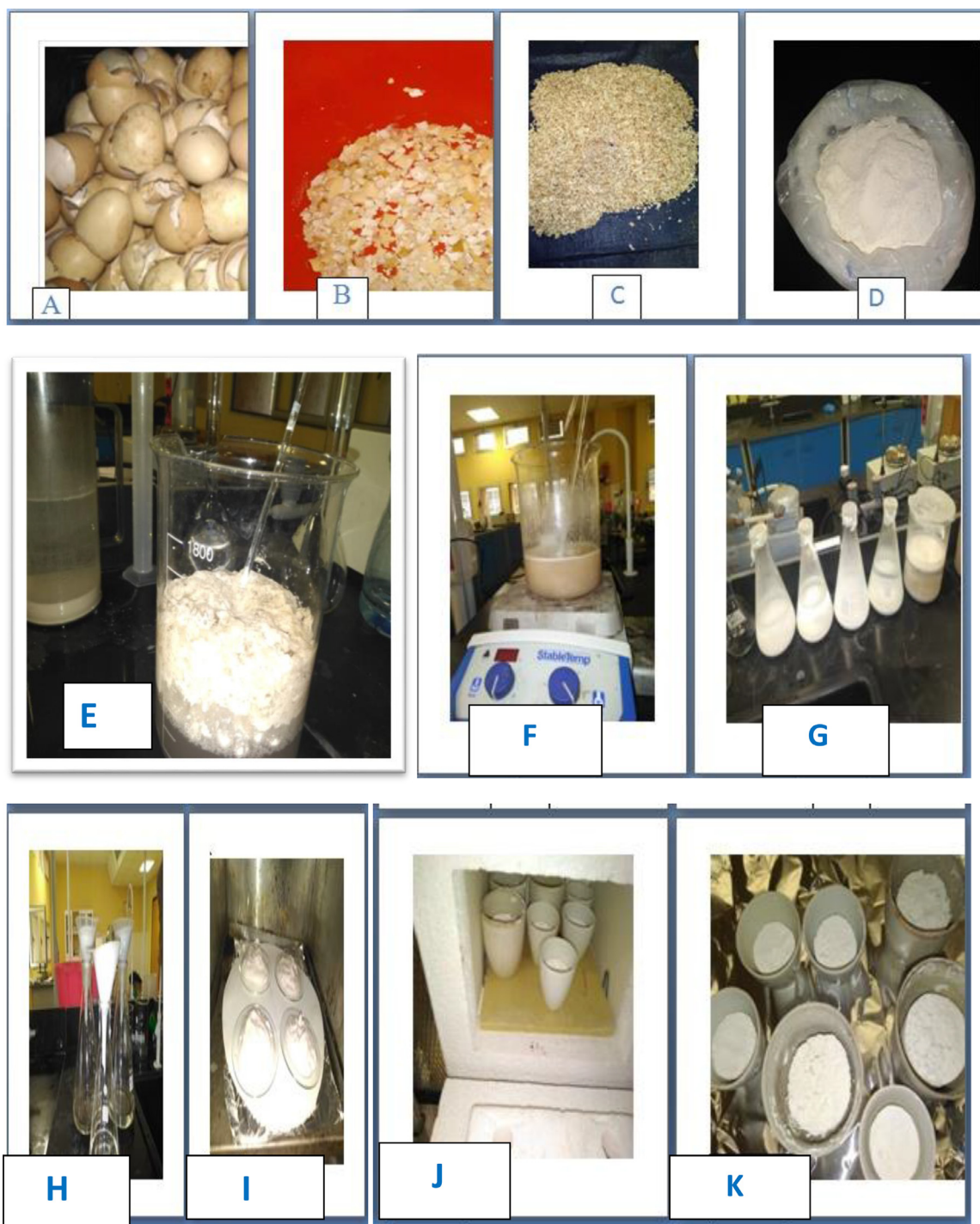
Fig. 1. Synthesis steps of CaO NP adsorbent A) Raw hen eggshells B) Washed hen eggshells C) Oven-dried eggshells D) sieved eggshells after ground E) preparation of homogeneous solutions F) Hydrolyses reaction G) condensation reaction H) Gel- filtration process I) Oven drying of Collection of filtered gels J) Muffle furnace calcination of dried gels K) Cancinated Gel powders (CaO NPs).
