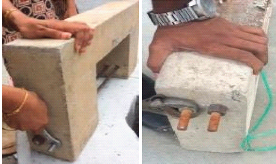
FIGURE 1: Formation of cracks due to stressing.
