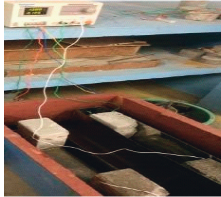
FIGURE 5: Accelerated corrosion test setup.
