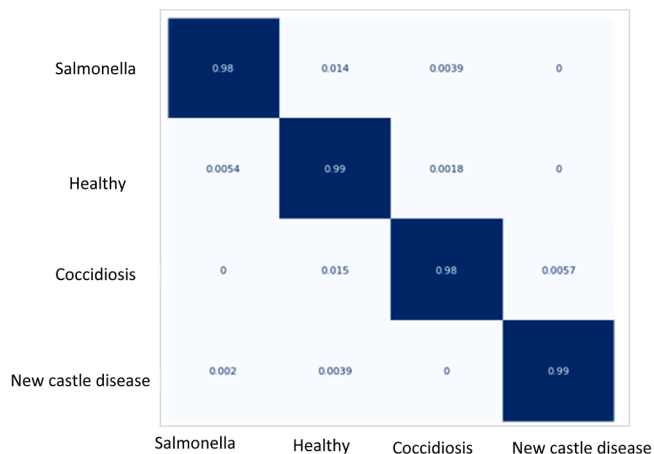
Fig. 11. Confusion matrix of the classifier. Y-axis represents the actual labels of the images while X-axis represents the labels as predicted by the classifier.
