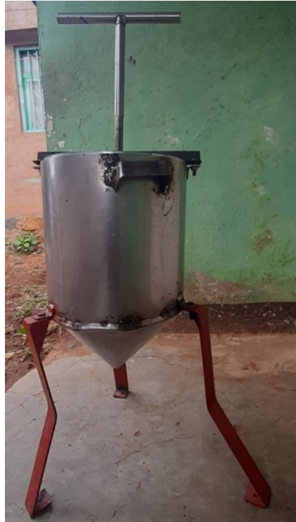
Figure 4 - 1 Developed Screw press honey extractor
