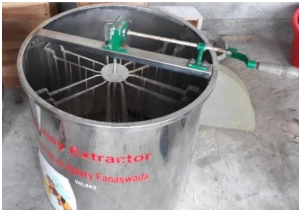
Figure 2 - 9 Manually-operated honey extractor
