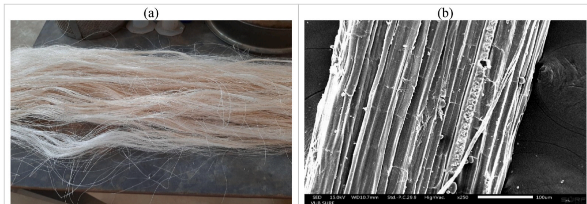
Fig. 1. a) Ensete Ventricosum (Ev) fibre bundles (approximately 45 cm long), (b) SEM surface observation.
