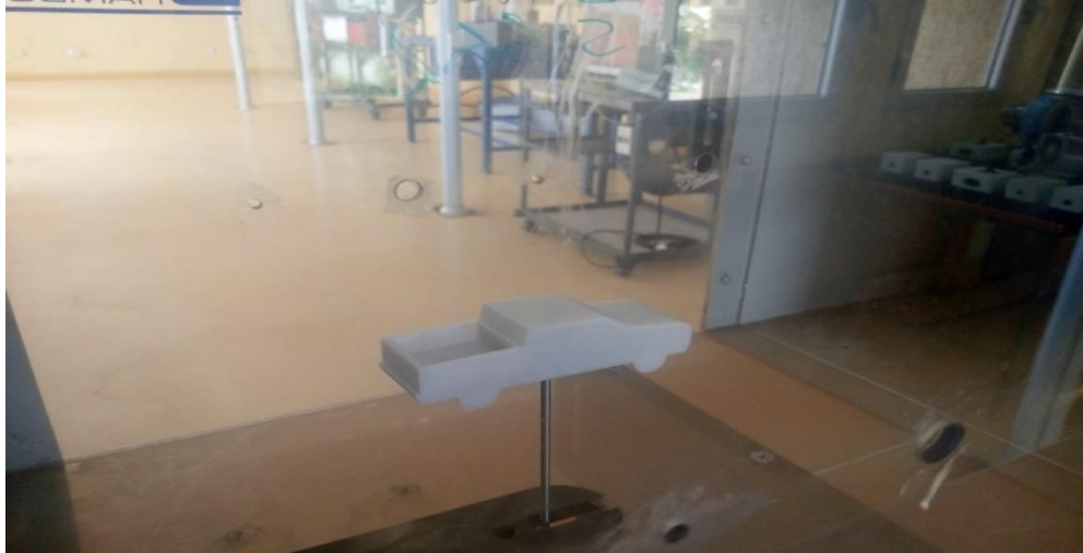
Figure 113: Installing the model into the wind tunnel machine
