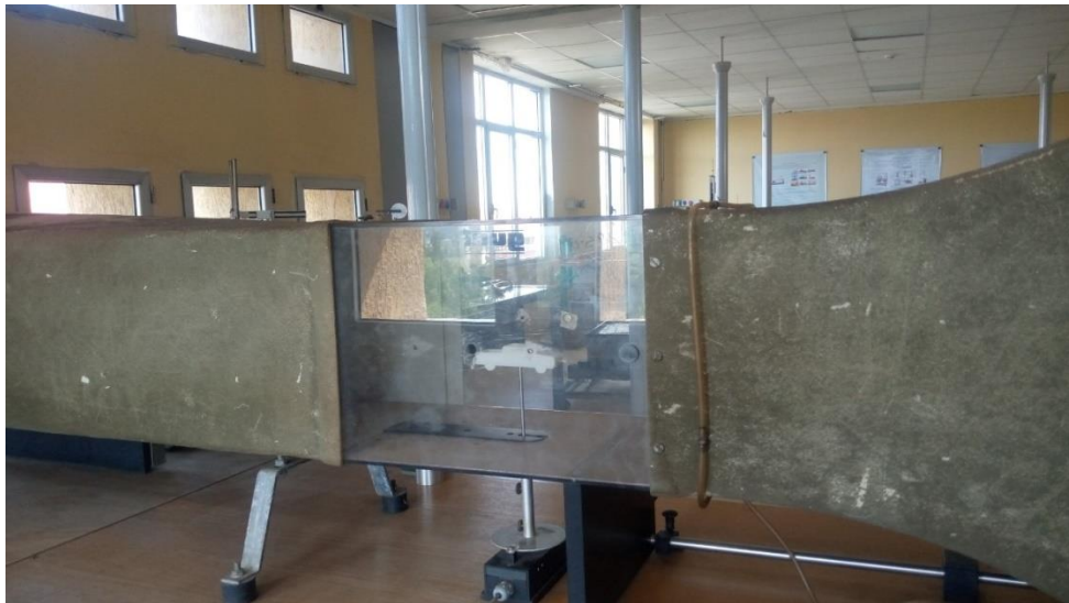
Figure 118: Scaled model during experimental test inside the wind tunnel test
