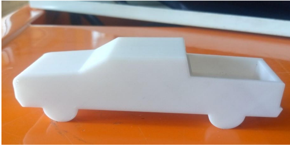
Figure 111: The 1/50 th scale model of Bishoftu double cabin pickup before an experimental test The 1/50 th scaled model of the Bishoftu double cabin pickup printed model is shown in Figure 111.
