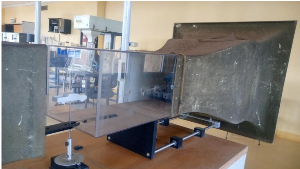
Figure 110: Wind tunnel structure in thermo fluid laboratory
