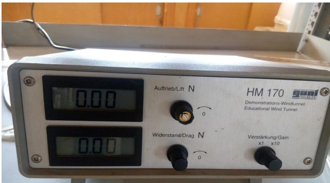
Figure 116: Digital amplifier for drag force (N) and lift force (N) measurements
