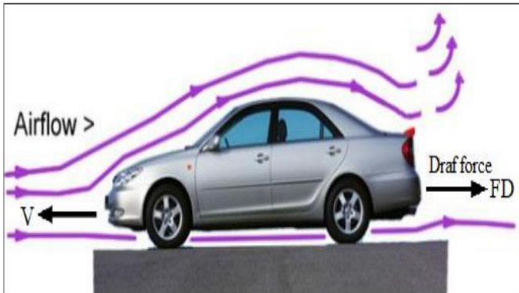
Figure 15: The drag force due to airflow acting on a car [44]
