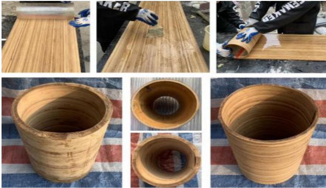
Figure 2.1: Manufacturing Process of The Bamboo Slices Twining Tube(Kou, Tian and Jin, 2021).
