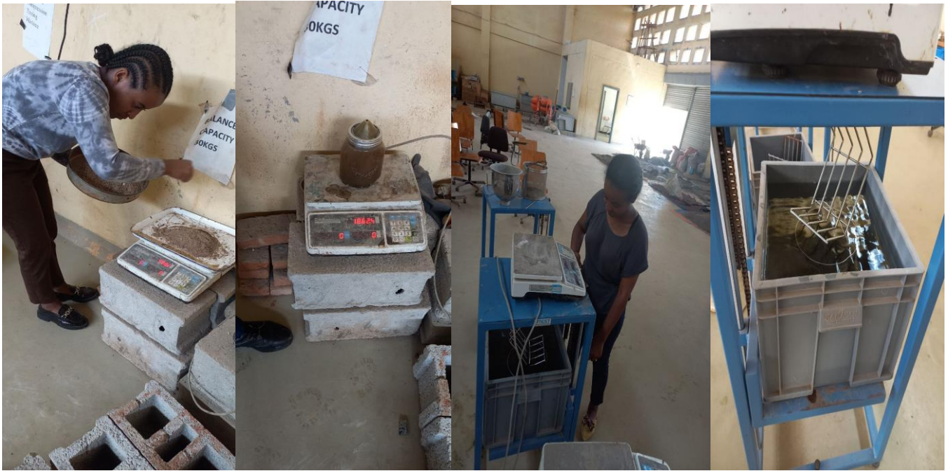
Photo-5 Specific gravity test for fine and coarse aggregate
