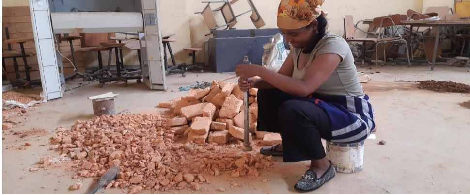
Figure 3-4 Size of manually crushed clay brick
