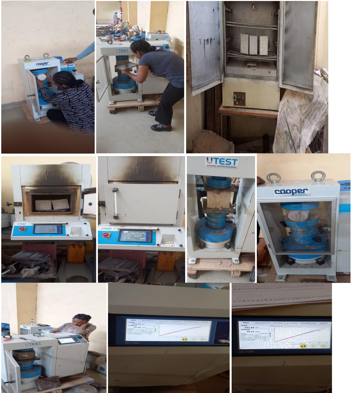
Photo-9 During hardened concrete test
