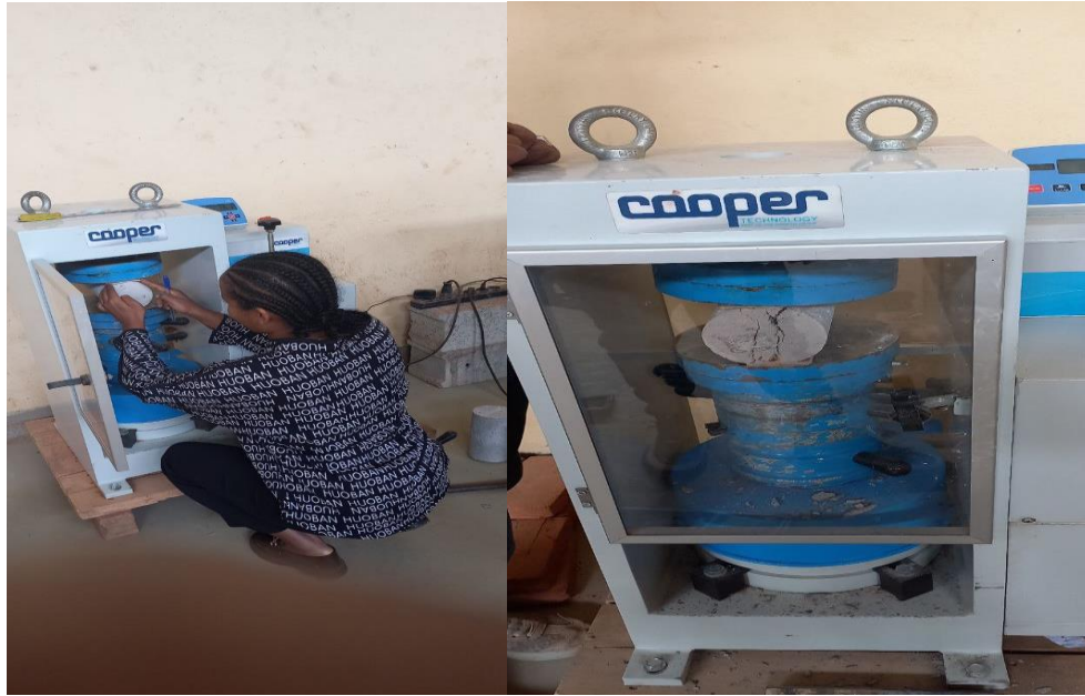
Figure 3-9 Split tensile strength test setup
