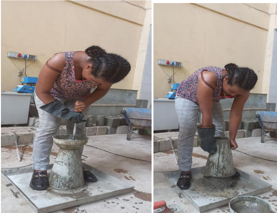
Photo-7 fresh concrete properties slump test
