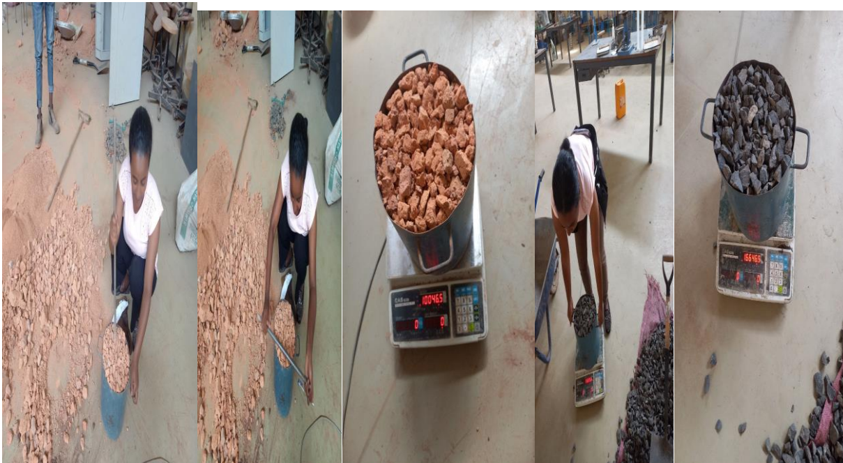
Photo-4 Unit weight of coarse aggregate
