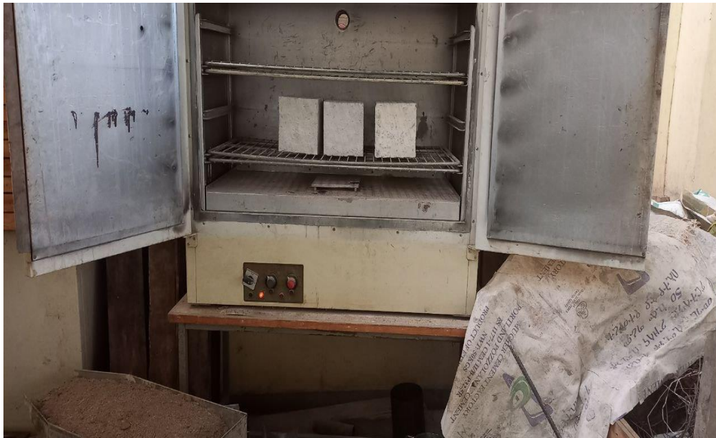
Figure 3-10 Water absorption test
