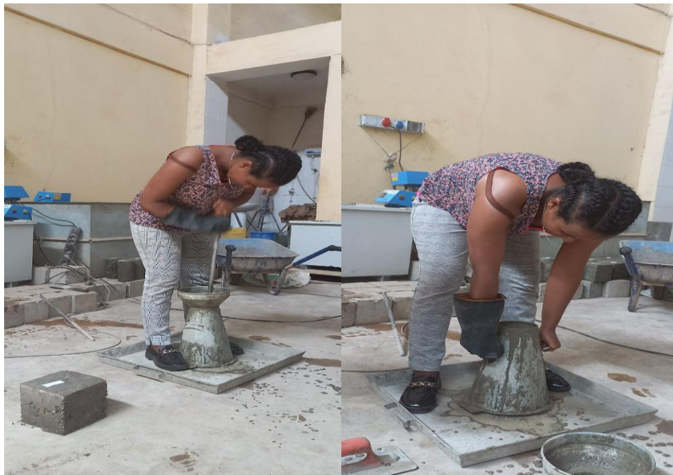
Figure 3-7 Slump cone test for the control mix
