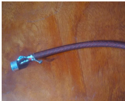
Figure 5.5: Illustration of the condenser microphone connected to an audio cable.
