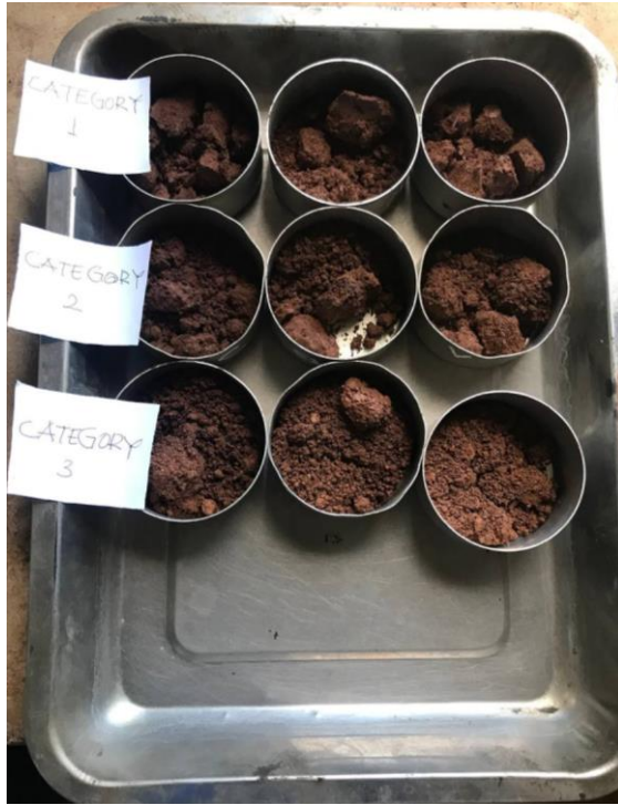
Moisture content determination
