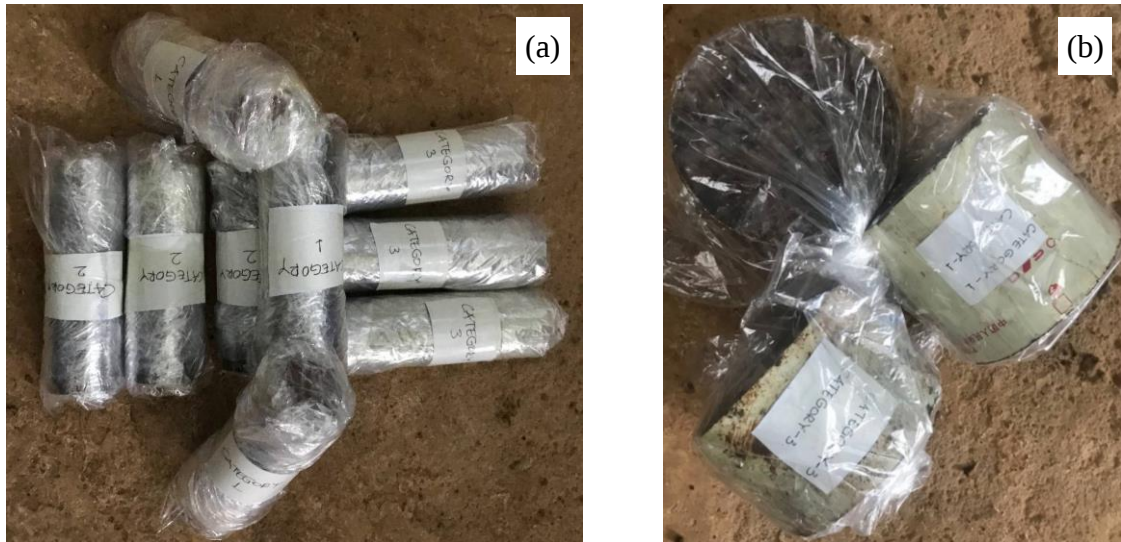
Figure 3-8 Waxed, labeled, and sealed undisturbed samples; (a) for triaxial compression test, and (b) for consolidometer test
