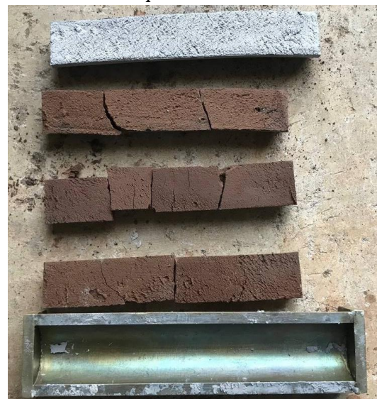
Linear shrinkage test
