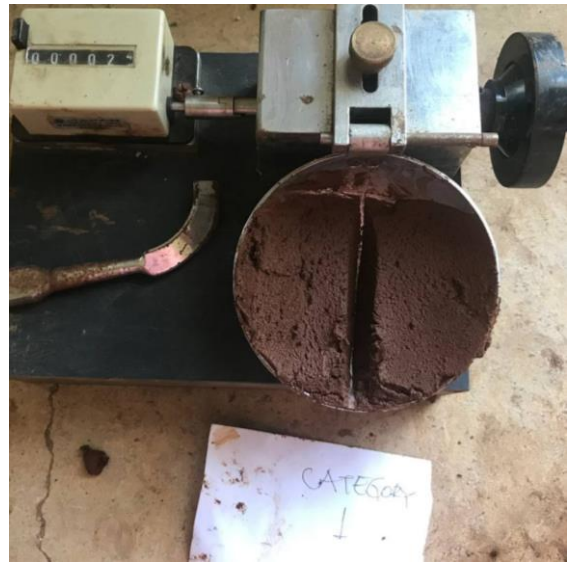
Liquid limit test
