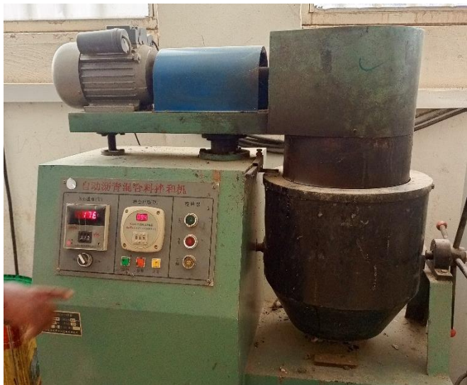
(1) Preheating aggregate at 175 °C
