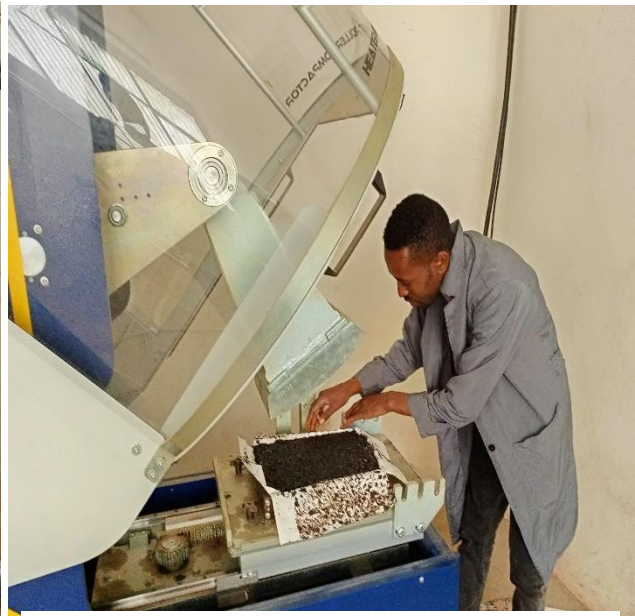
(4) Sample under roller asphalt compactor
