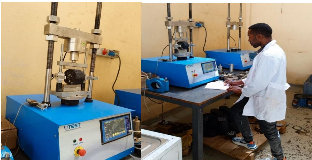
Figure 3.10: Indirect tensile strength test
