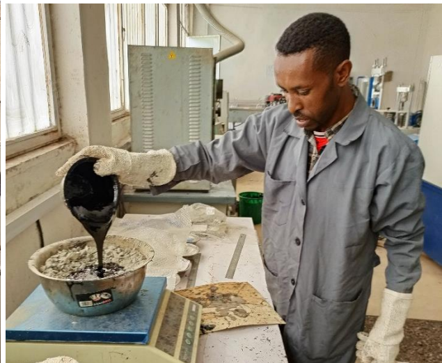
(2) Add heated bitumen to preheated aggregate
