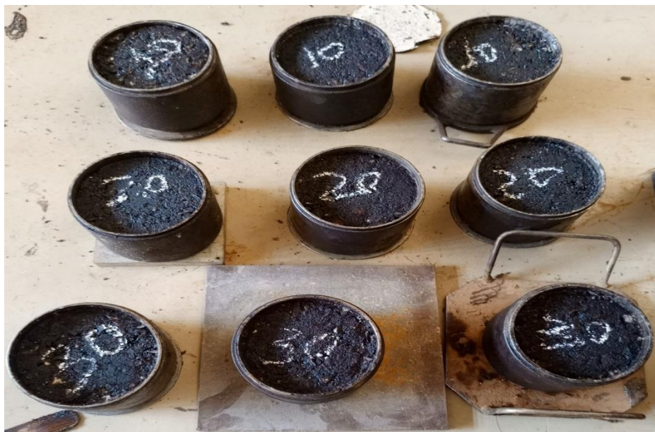
Figure 3.8: Waste marble modified Marshall specimen
