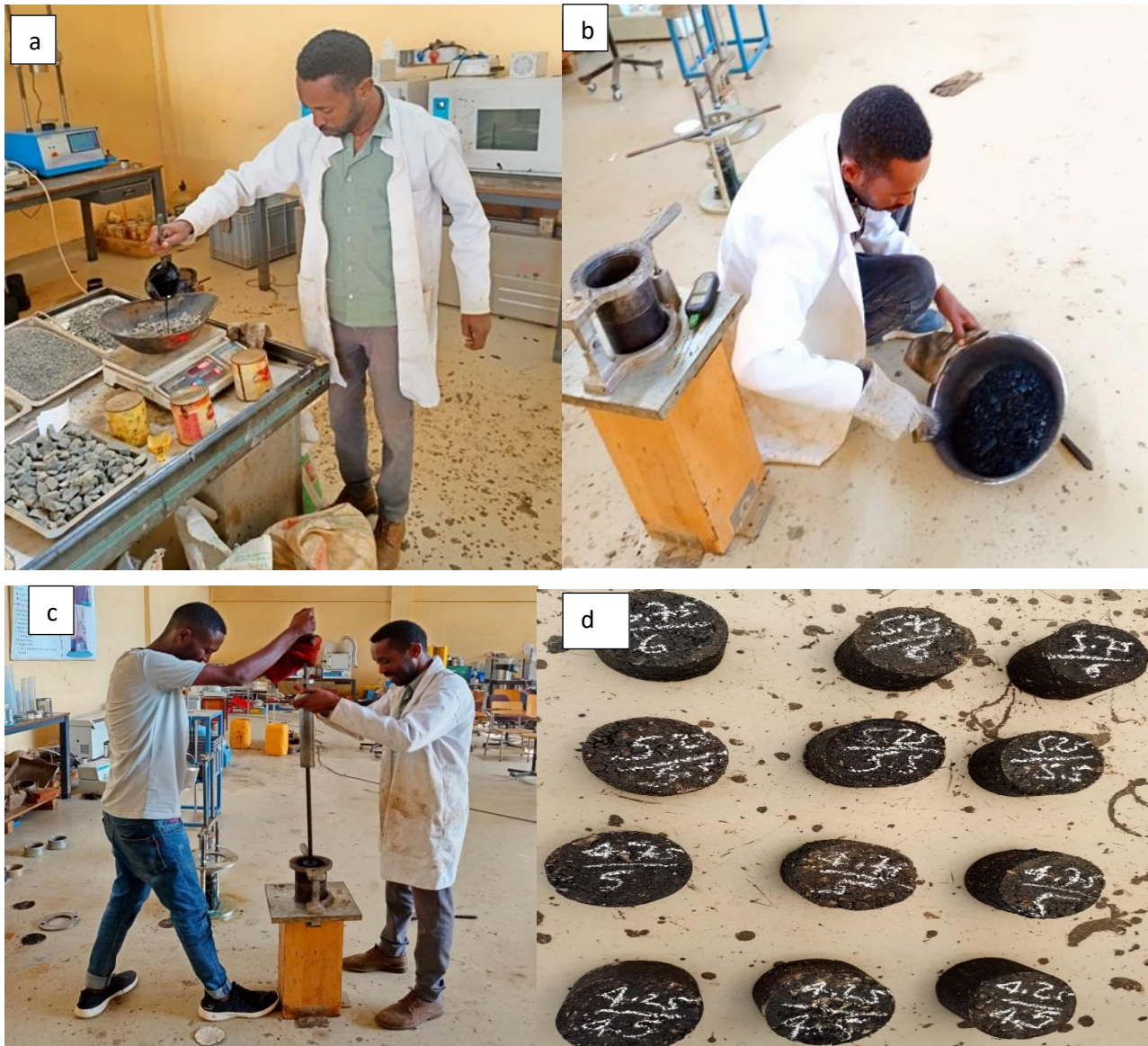
Figure 3.4: Marshall specimen preparation (a) pouring the heated bitumen to aggregate, (b) mixing, (c) compact and (d) compacted Marshall specimen
