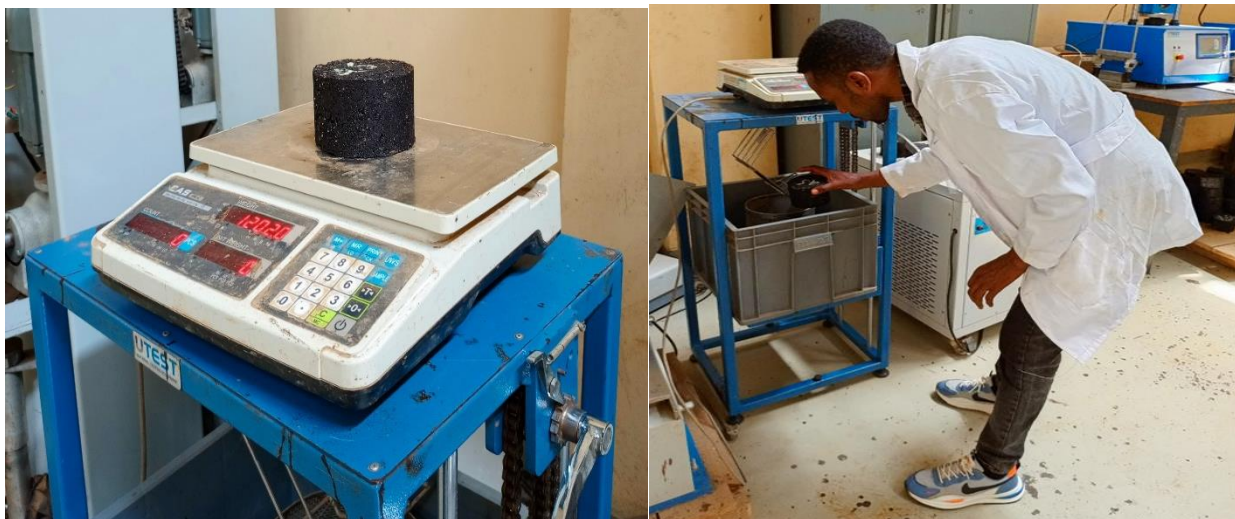
Figure 3.5: Bulk specific gravity test
