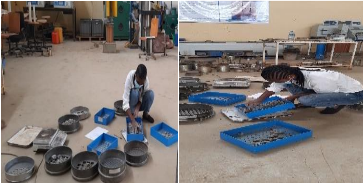
Figure 3. 3 Photos while conducting Flakiness and Elongation Tests
