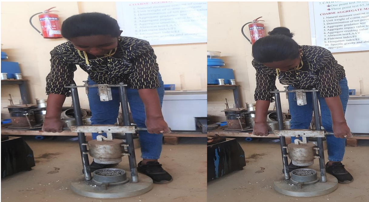
Figure 3. 8 Photos during performing Aggregate Impact Value
