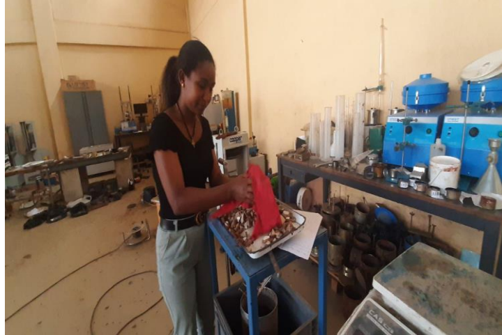
Figure 3. 6 Photos while conducting Specific gravity and water absorption
