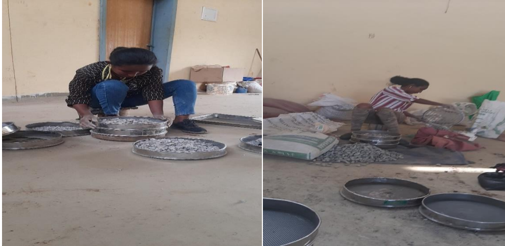
Figure 3. 4 Photos while conducting a gradation test
