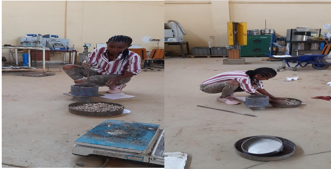
Figure 3. 7 Photos during performing Aggregate crushing value
