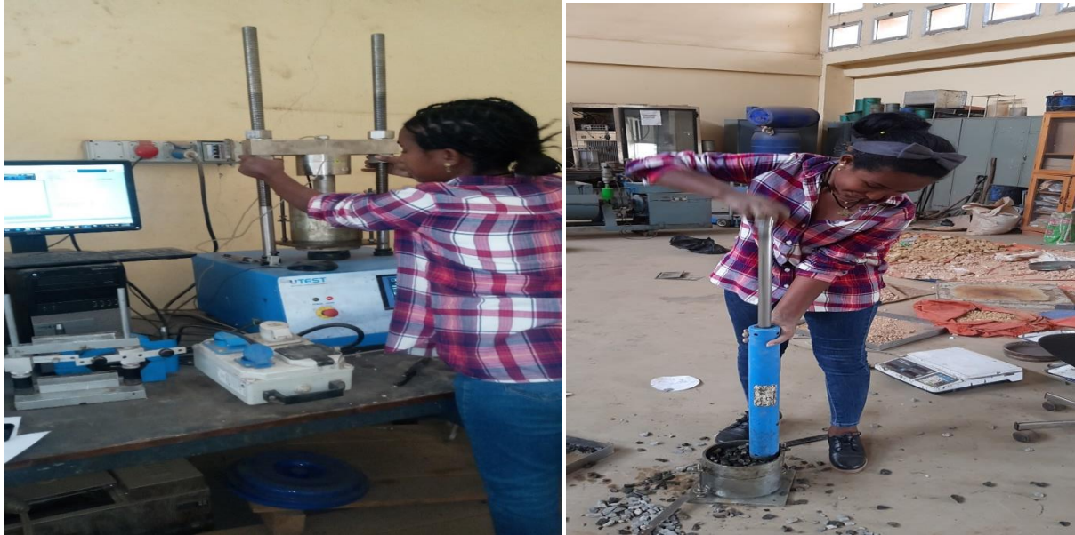
Figure 3. 10 Photos during performing CBR tests
