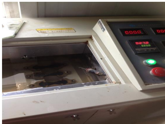
Figure 3.14: Ductilometer test setup.
