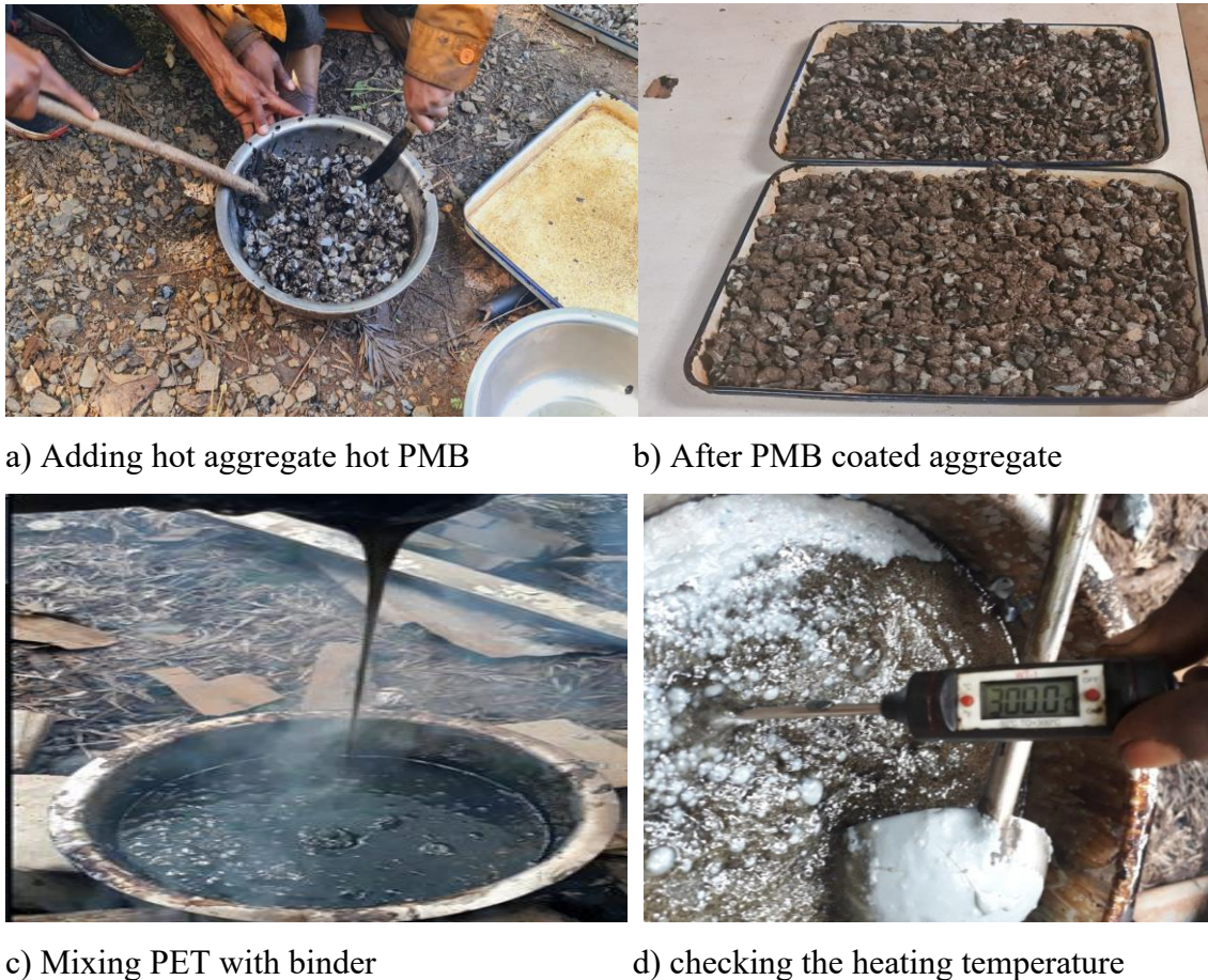
Figure 3.7: Waste plastic Coated aggregate sample preparation (a, b, c and d).
