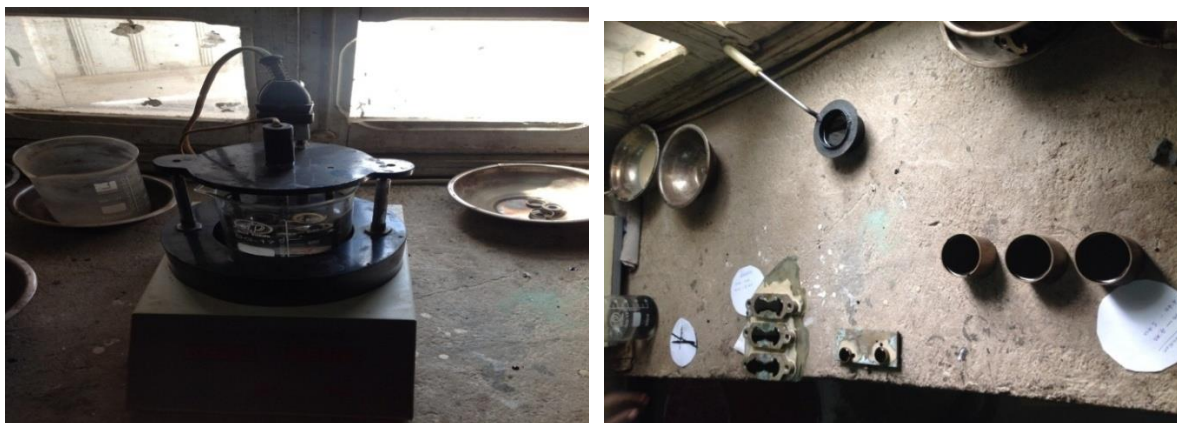
Figure 3.13: Softening point ring and ball apparatus setup.
