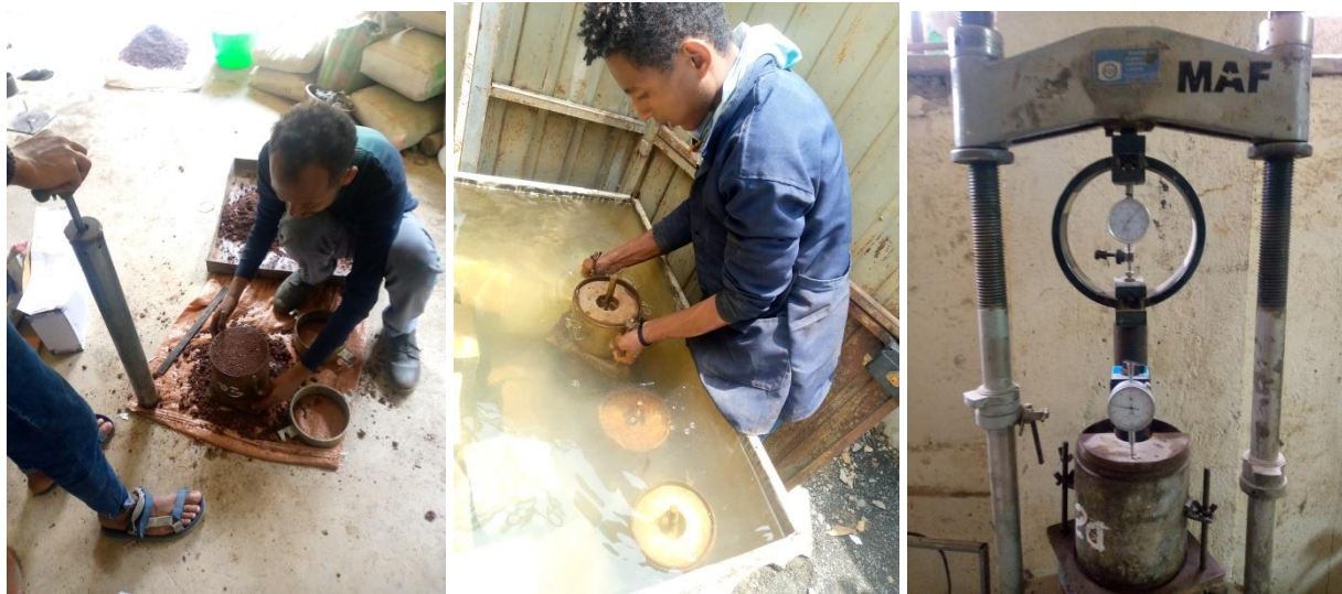
Figure 3.11: CBR test procedures
