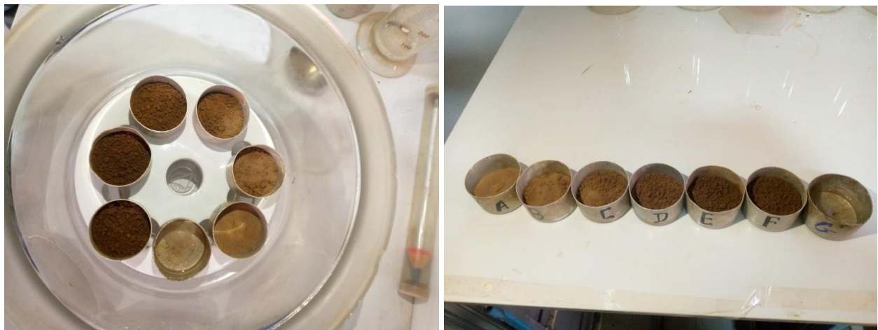
Figure 3.6 (c): Moisture absorption/hygroscopicity test, after 7 days
