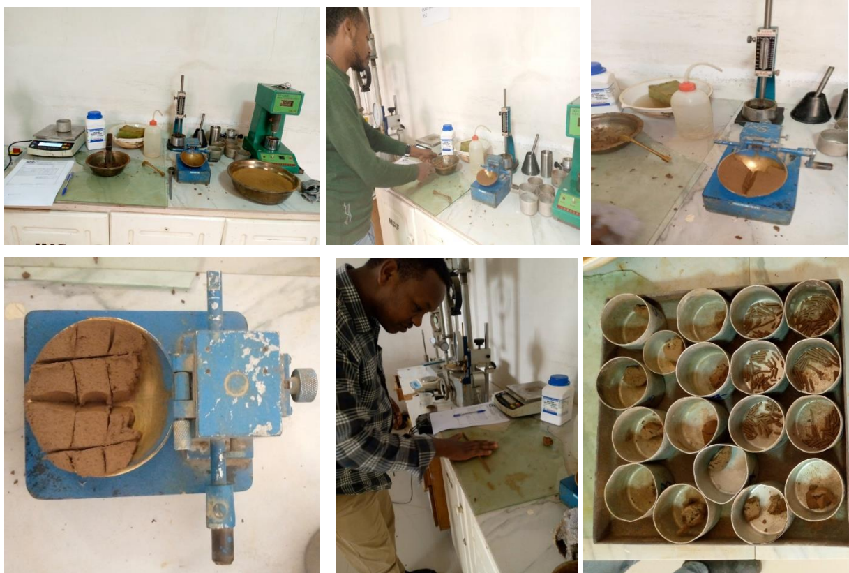
Figure 3.7: Atterberg limits determination
