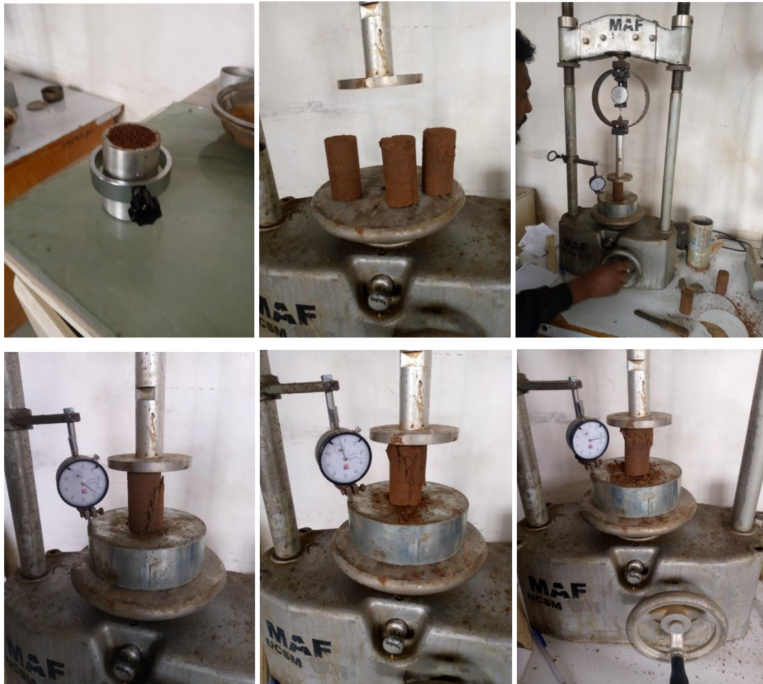
Figure 3.10: Unconfined compression test
