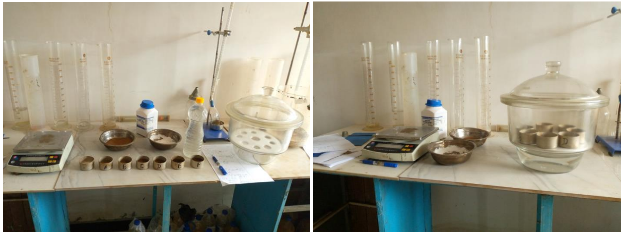
Figure 3.6 (a): Moisture absorption/hygroscopicity test
