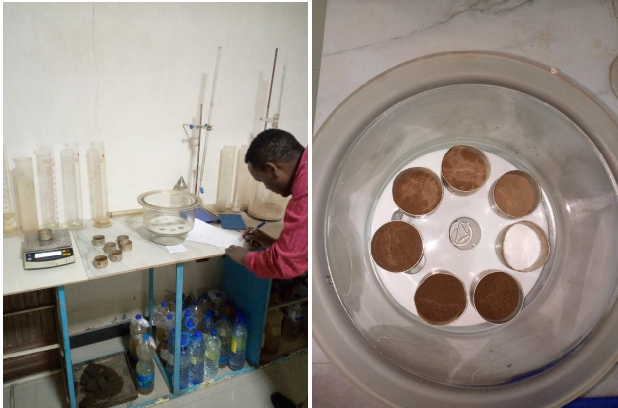
Figure 3.6 (b): Moisture absorption/hygroscopicity test, after 24 Hours
