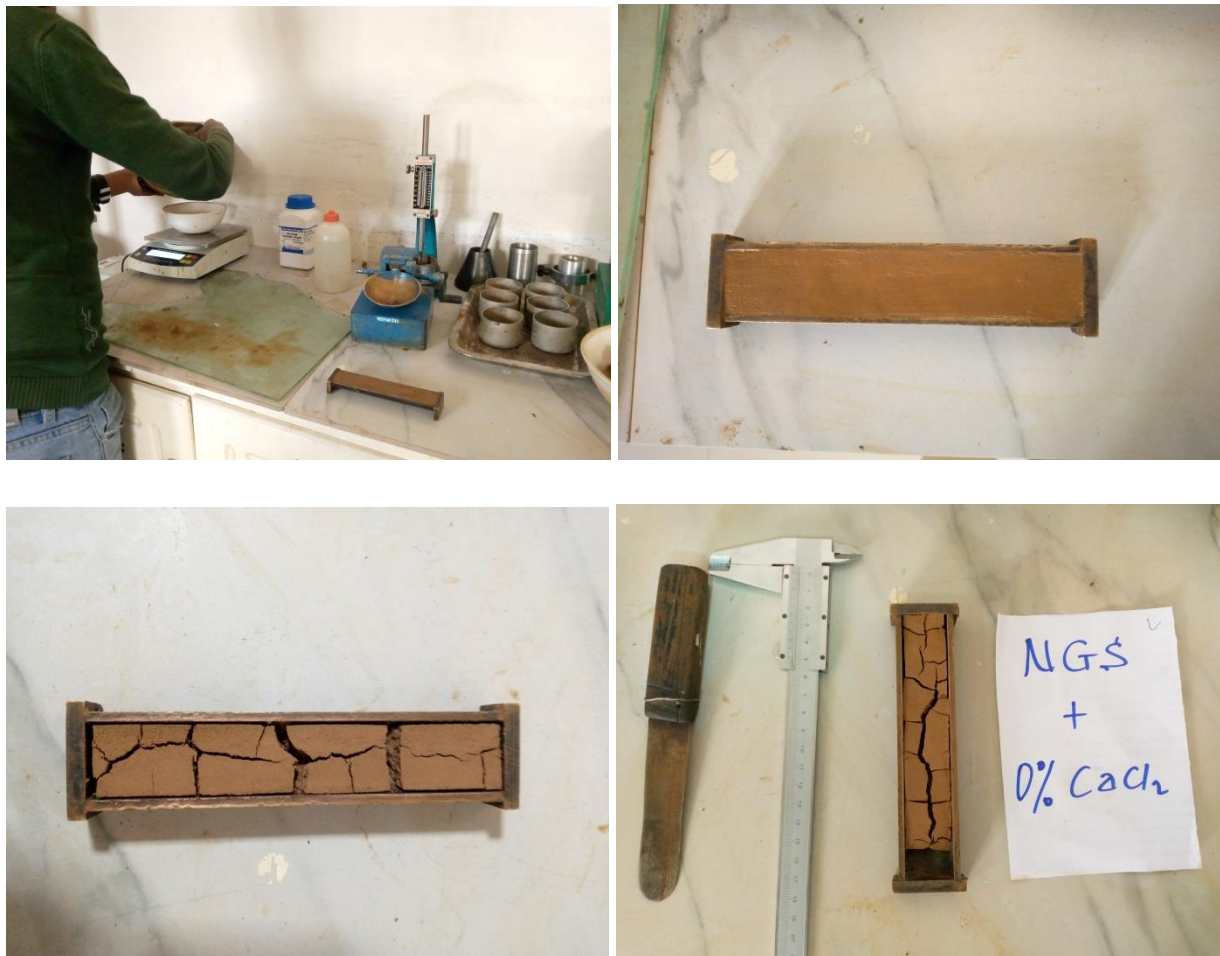
Figure 3.8: Linear shrinkage test
