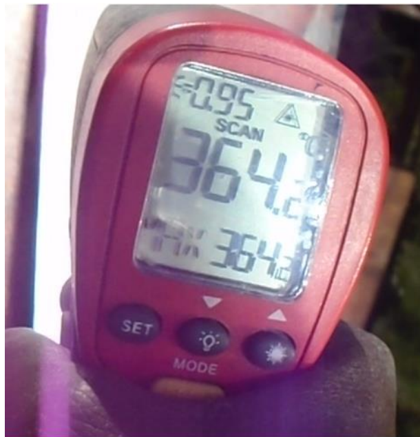
Photo shows temperature obtained in flat iron during testing without oven
