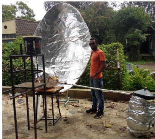
Fig. 12. System component of Scheffler reflector solar sesame oil distiller
