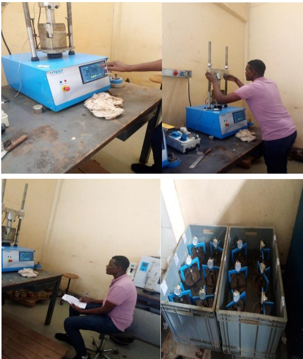
Figure 3.9: CBR test photos (captured by Gizaw)
