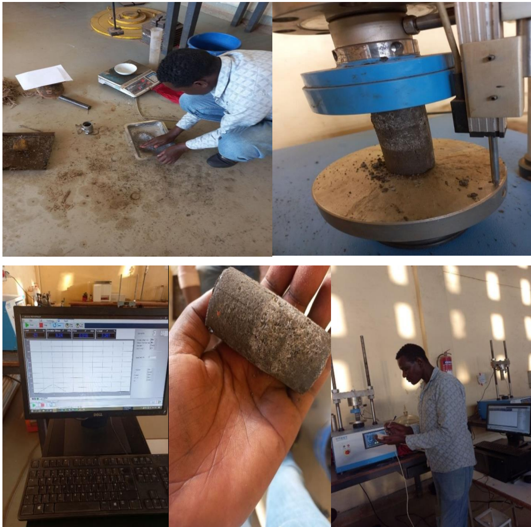
Figure 3.10: UCS test photos (captured by Haile)
