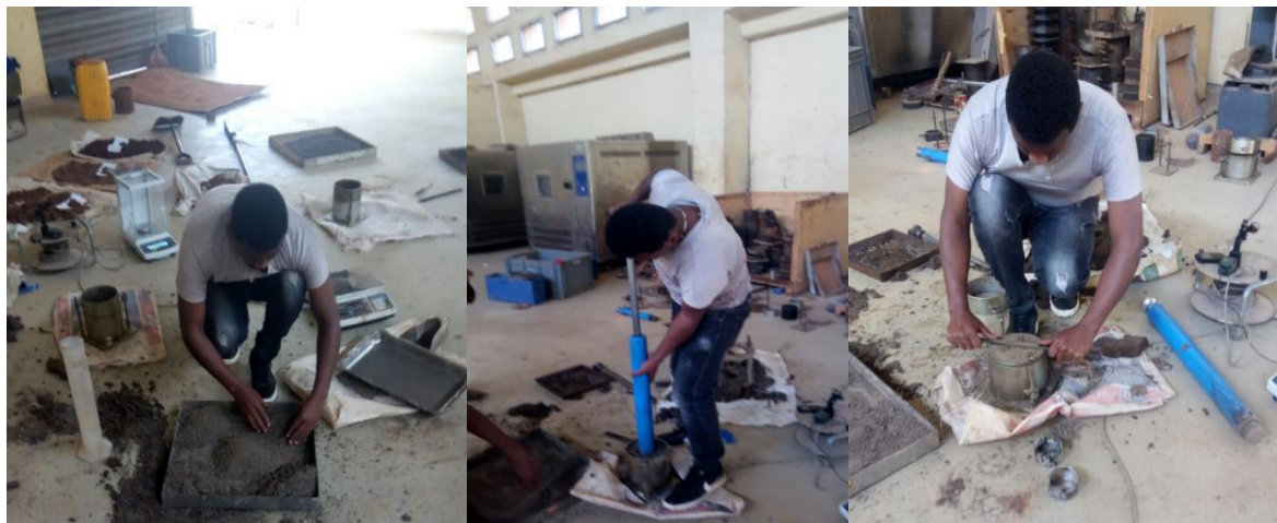
Figure 3.11: Compaction test Procedure (photo captured by Mohammed N.)
