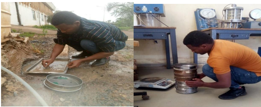
Figure 3.9: Particle size distribution test (photo captured by Mohammed N.)
