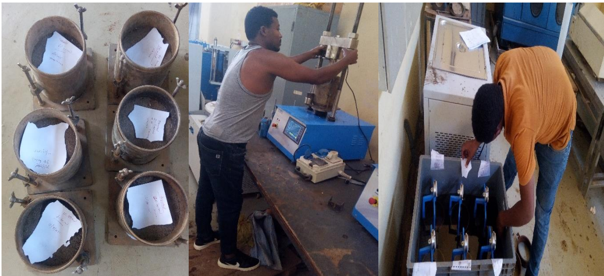
Figure 3.12: CBR and CBR-swell test (photo captured by Giza T.)
