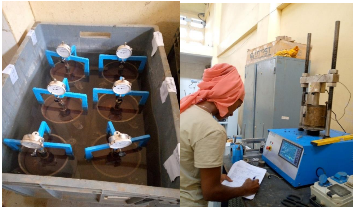
Figure 3.9: California Bearing Ratio (CBR) And CBR Swell
