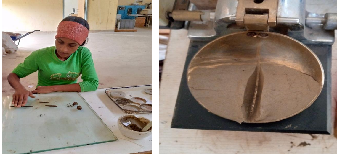
Figure 3.5: Liquid Limit and Plastic Limit Determination
