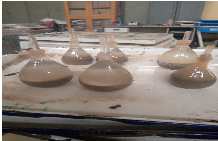
Figure 3.7: Specific Gravity Determination
