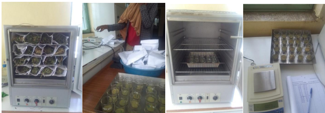
DM Determination (DM% were determined for 24hrs at 105 °C both for forage and silage)
