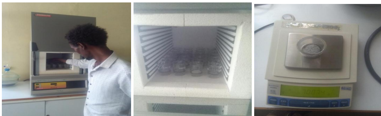
Ash determination both for forage and silage at 500 °C for 3hrs.
