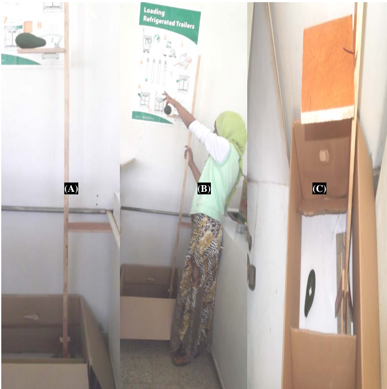
Appendix figure 2. Fruit ready to drop from the height of 1.58m on the prepared stationary pole (A) Allowing the fruit to fall freely on the height of 1.58m from the stationary pole (B) fruit bounded and fruit failed after drop treatment of the assigned height (C)
