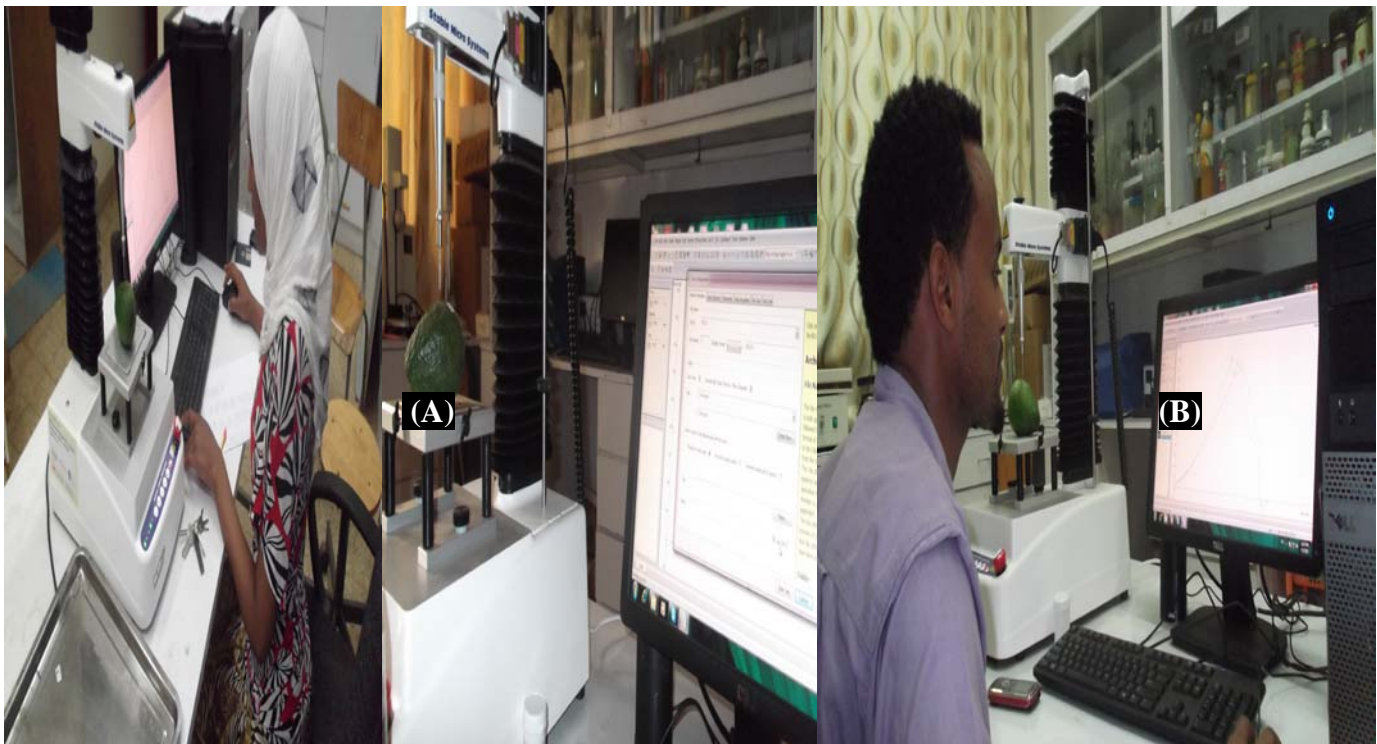
Appendix Figure 9. Testing of avocado fruits using computerized TA-XT plus software (A) and (C) output readings noted on the computer reading chart, to one decimal place(B)
